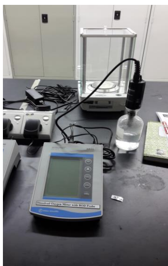
Figure 3.5: DO meter (Fisher Scientific, acumet AB40)
