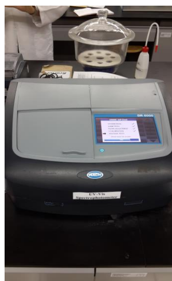
Figure 3.8: UV-Vis-Spectrophotometer (Hach, DR 6000, USA)
