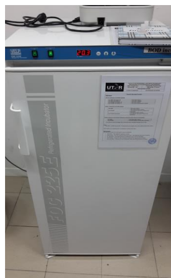
Figure 3.6: BOD incubator (VELP Scientifica, FOC 225E)
