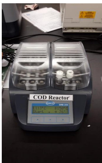
Figure 3.7: COD reactor block (Hach, DRB 200, USA)
