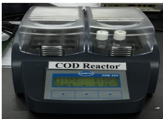
Figure 3.5 COD Reactor Block (DRB 200, USA)
