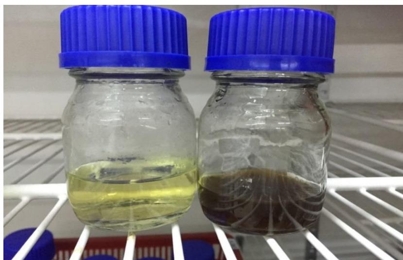
Figure 4.11 Comparisons between Treated (Left) and Non-Treated (Right) POME Sample Using Electro Oxidation Process
