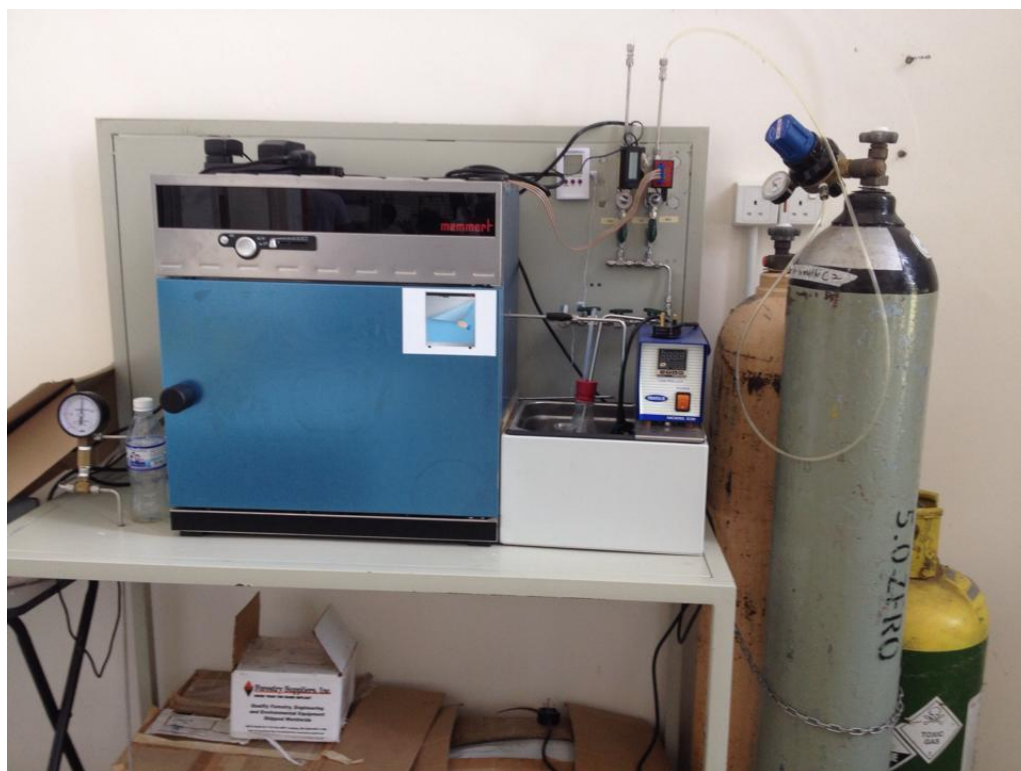
Figure 3.2 The apparatus setup for the sulphur dioxide test
