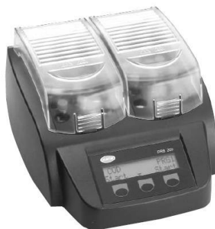
Figure 3.3: COD Reactor Hach DRB-200
