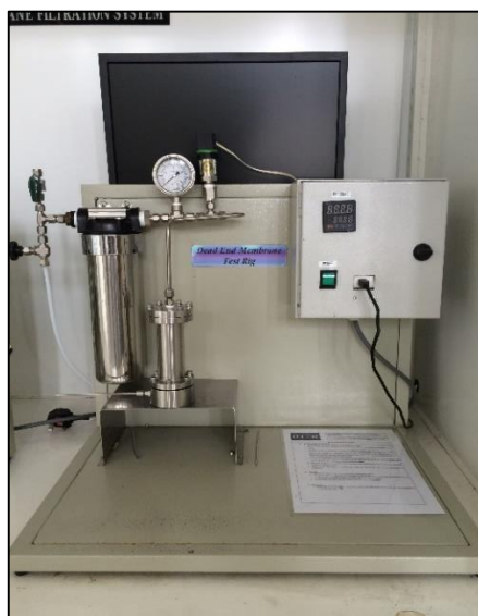
Figure 3.9: Dead End Membrane Test Rig
