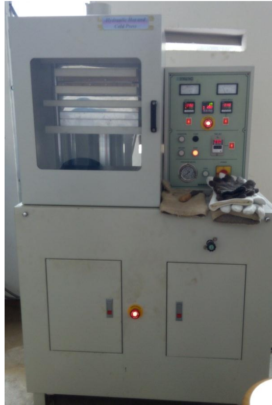
Figure 3.4: Hydraulic Hot and Cold Press Machine
