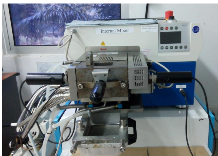
Figure 3.3: Brabender® Plastograph® EC 815652 Internal Mixer
