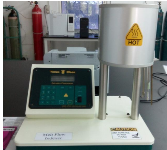
Figure 3.5: Tinius Olsen Extrusion Plastometer model MP600
