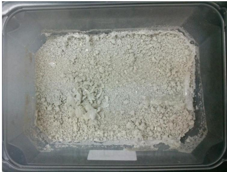
Figure 4.3: Epoxy mixture: water ratio, 60g: 120g
