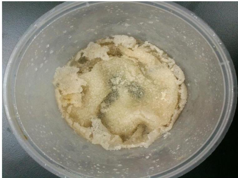
Figure 4.5: Epoxy mixture: water ratio, 60g: 140g
