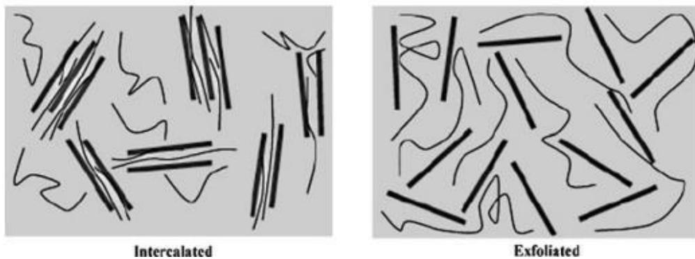
**Figure 2.5 types of morphologies structure**
