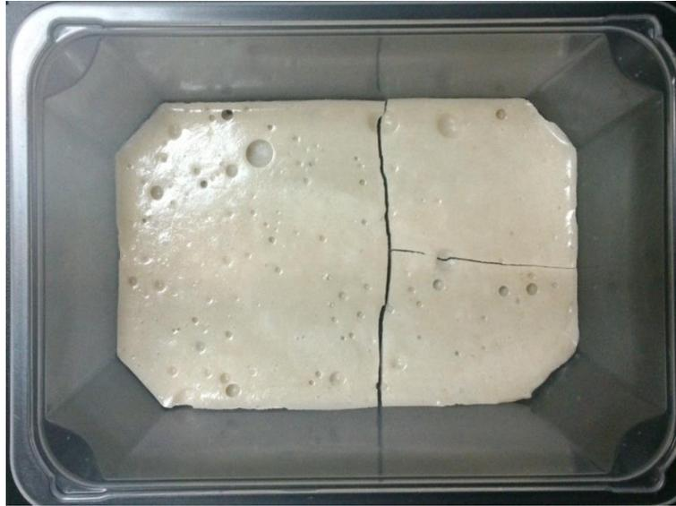
Figure 4.2: Epoxy mixture: water ratio, 60g: 110g
