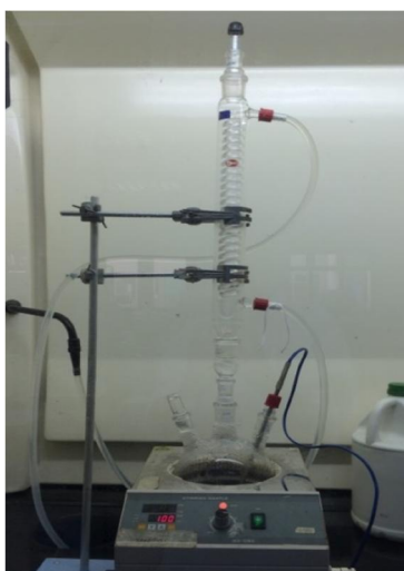
Figure 3.4: Experimental Setup for Preparation of RGO
