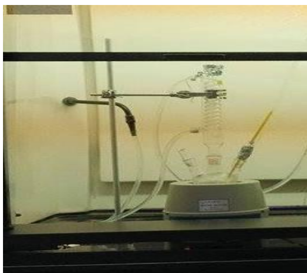
Figure 3.1: Reflux Condensation Set Up
