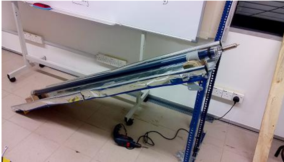
Figure 6: Photograph of installation heat pipe with metal frame
