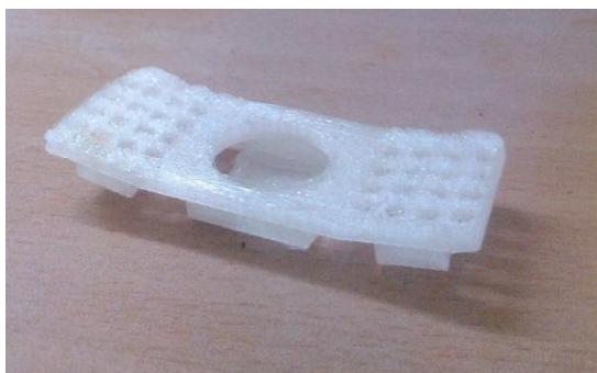
Figure 4.16: The chin guard printed by 3D printer
