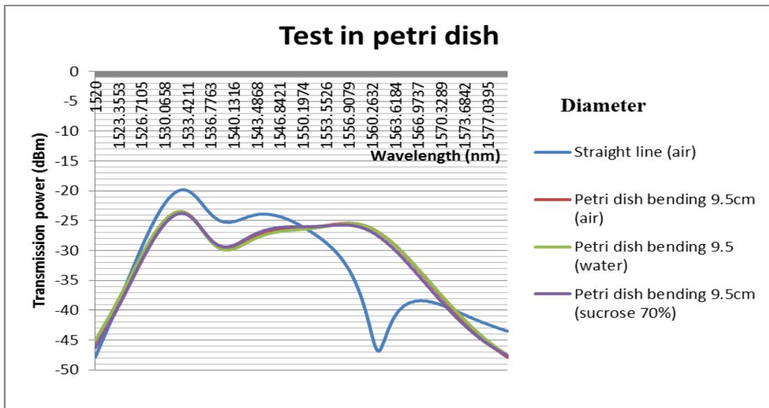
Figure 4.3-17: The weight with 14g and 40 number of grating period fiber was tested in petri dish
