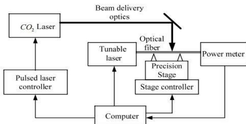
Figure 2.2-1: Schematic setup of the CO<sub>2</sub> laser based LPFG fabrication system
