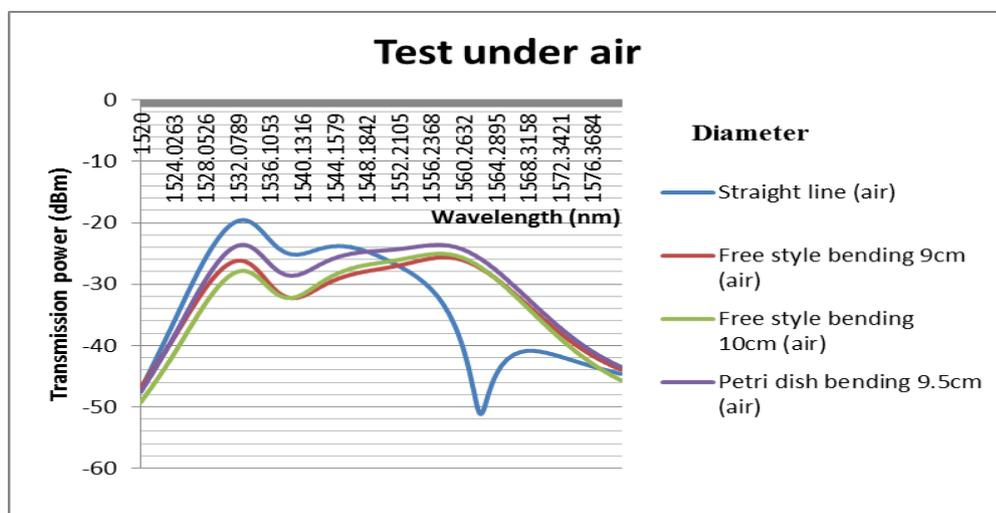
Figure 4.3-7: The weight with 14g and 29 number of grating period fiber was tested under air condition with different bending structures
