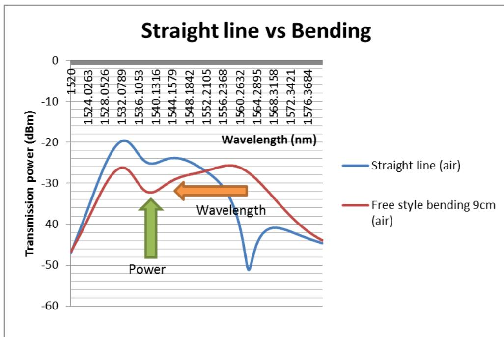
Figure 4.3-8: Comparison between straight with bending method. Power was drop from -51.163dBm to -32.271dbm. Wavelength was shift 23.506nm to left side
