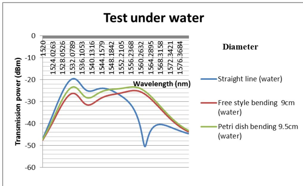
Figure 4.3-9: The weight with 14g and 29 number of grating period fiber was tested under water condition with different bending structures
