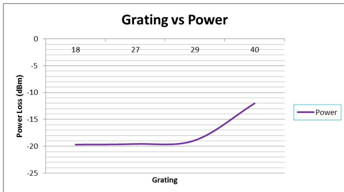
Figure 4.4-1: Power loss has been measure from straight line to bending method in different grating. More grating has lower transmission loss
