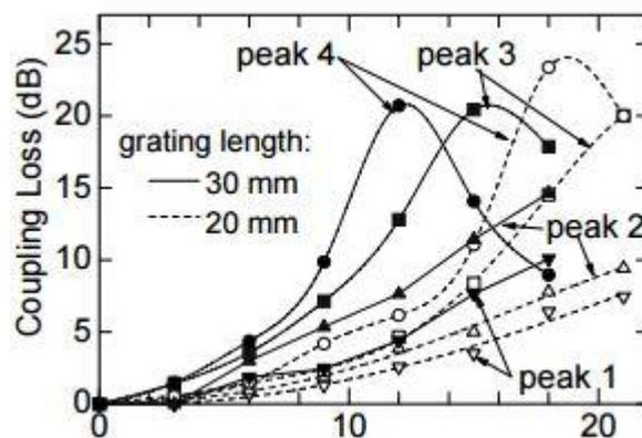
Figure 2.4-3: Growth characteristics of resonance peaks of LPGs with a grating period of  $212\mu\text{m}$ .
