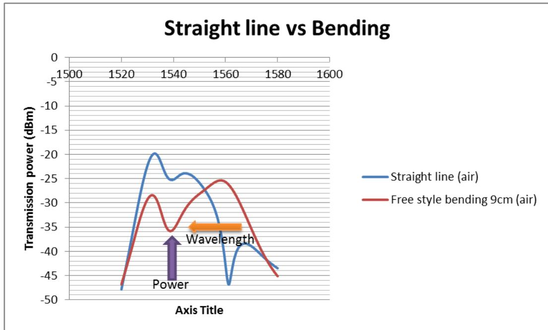
Figure 4.3-14: Comparison between straight with bending method. Power was drop from -46.855dBm to -35.826dbm. Wavelength was shift 22.342nm to left side
