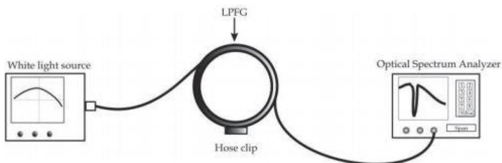
Figure 2.1-3: Experimental setup for sensing diameter of curvature (Estudillo-Ayala, 2011)
