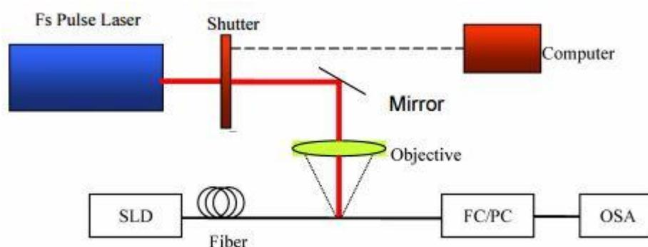
Figure 2.3-1: The experimental setup for LPFG fabrication technique by Femtosecond Laser (Kondo, 2011)
