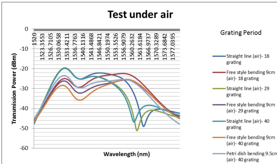
Figure 4.4-3: The number of 18, 29 and 40 grating has used to test under air condition in straight line and bending method
