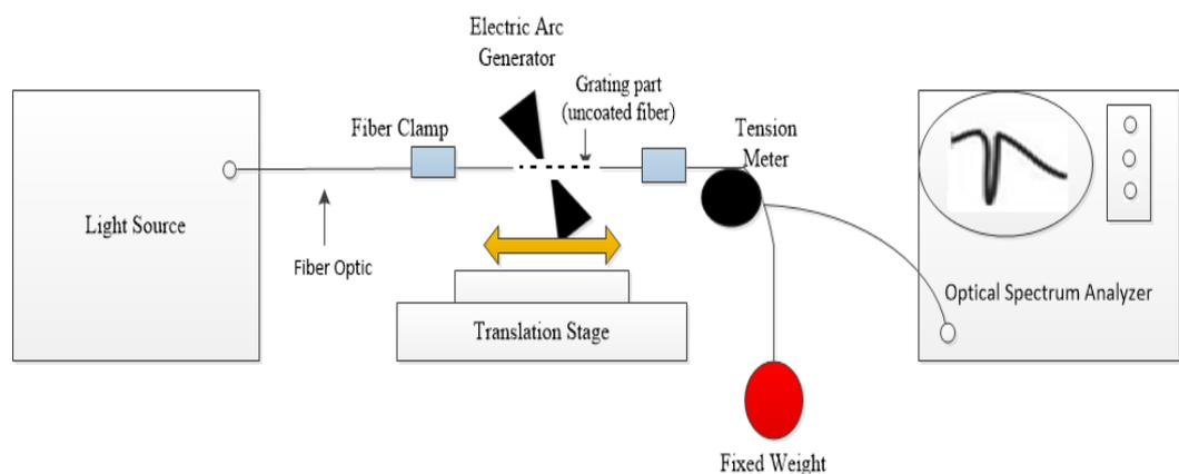
Figure 3.2-1: Experimental Setup of LPFG fabricated by electric arc
