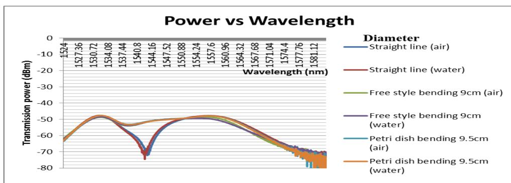
Figure 4.7-1: Fiber with 57 grating period with 22g test under air and water condition with different bending structures
