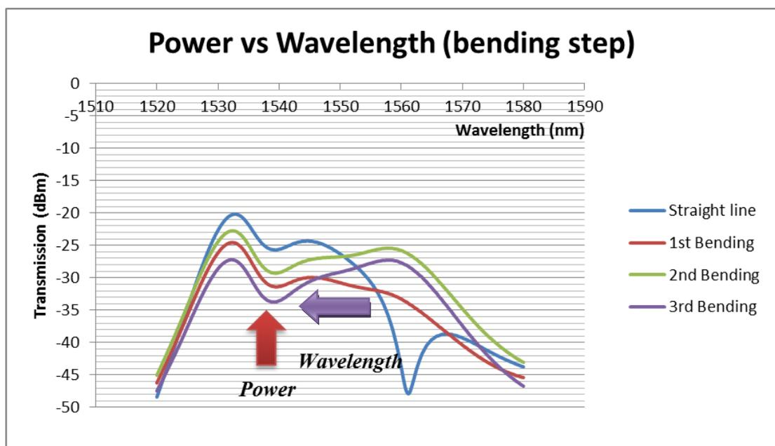
Figure 4.2-1: Bending step waveform. After implement with bending method which the wavelength has shifted to left and the power has move to upward
