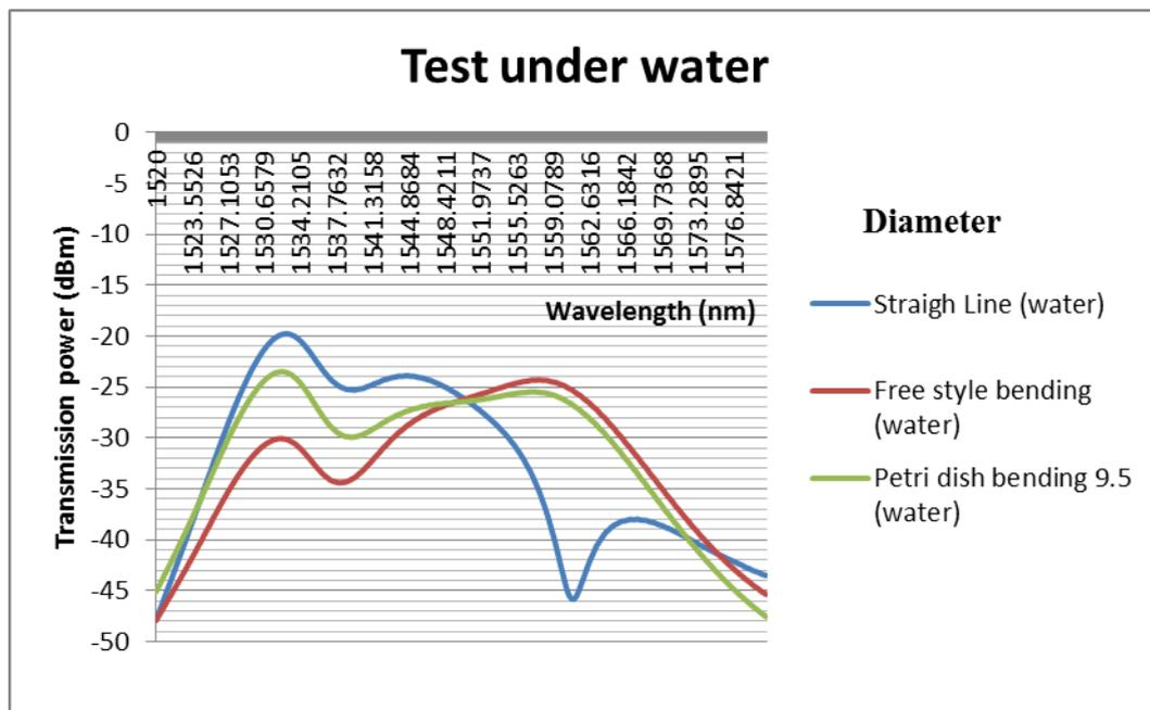
Figure 4.3-15: The weight with 14g and 40 number of grating period fiber was tested under water condition with different bending structures
