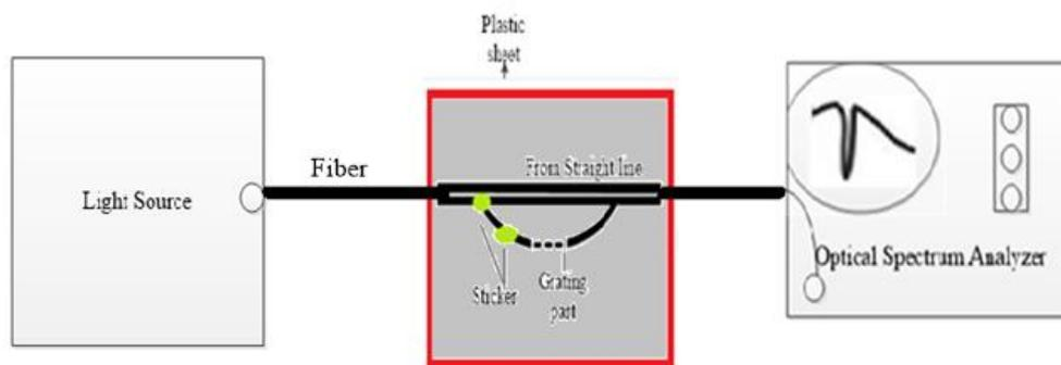
Figure 3.2-3: Experimental Setup for bending structure in plastic sheet
