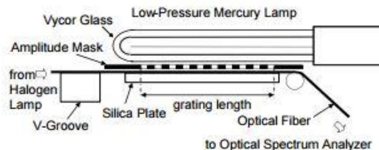
Figure 2.4-1: The experimental setup for fabrication LPFGs by mercury-lamp exposure (Mizunami, 2014)
