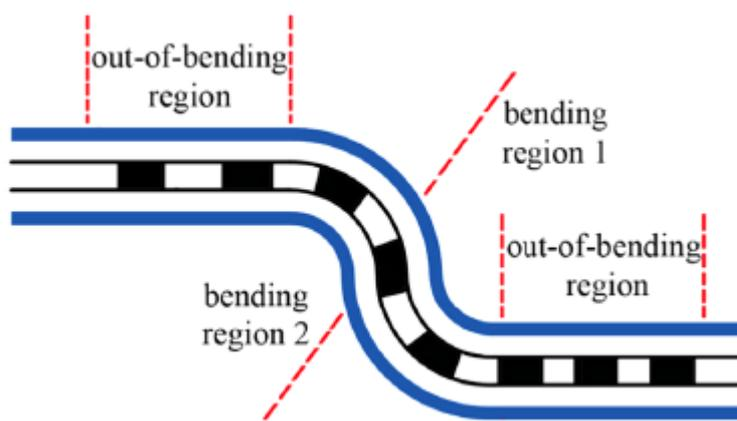
Figure 2.5-1: The structure bending in a LPFG-based bending sensor (Taghipour, 2014).
