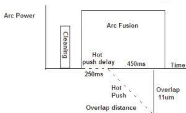
Figure 2.1-6: Time delay of the standard discharged method
