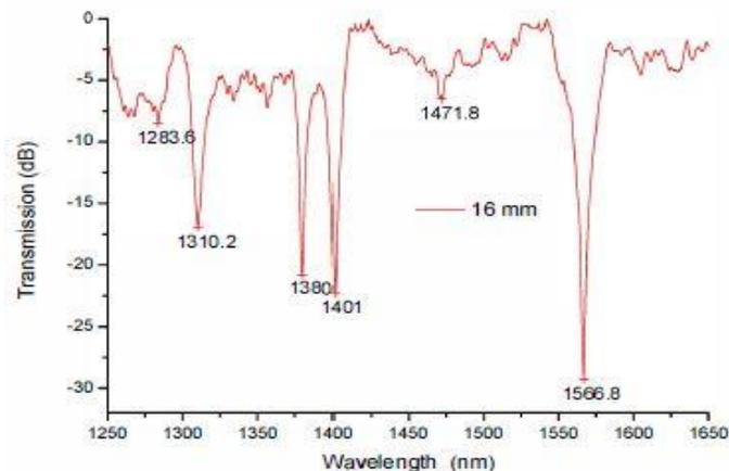
Figure 2.3-2: The transmission spectrum of LPFG with grating period of 400  $\mu\text{m}$  and length of 16 mm
