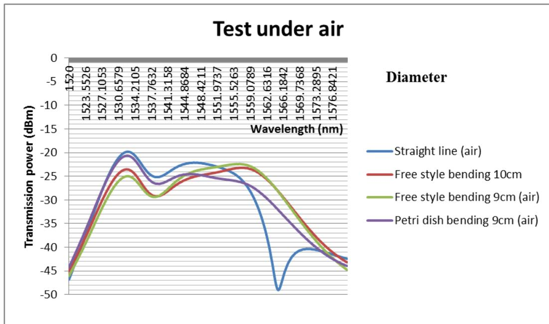
Figure 4.3-1: The weight with 14g and 18 number of grating period fiber was tested under the air condition with different structures
