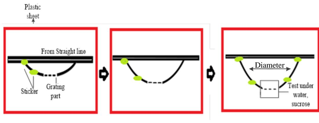
Figure 3.2-4: The experiment setup for the free style bending step. The notch was obtained in the right side picture so use that structure to test under water and sucrose condition
