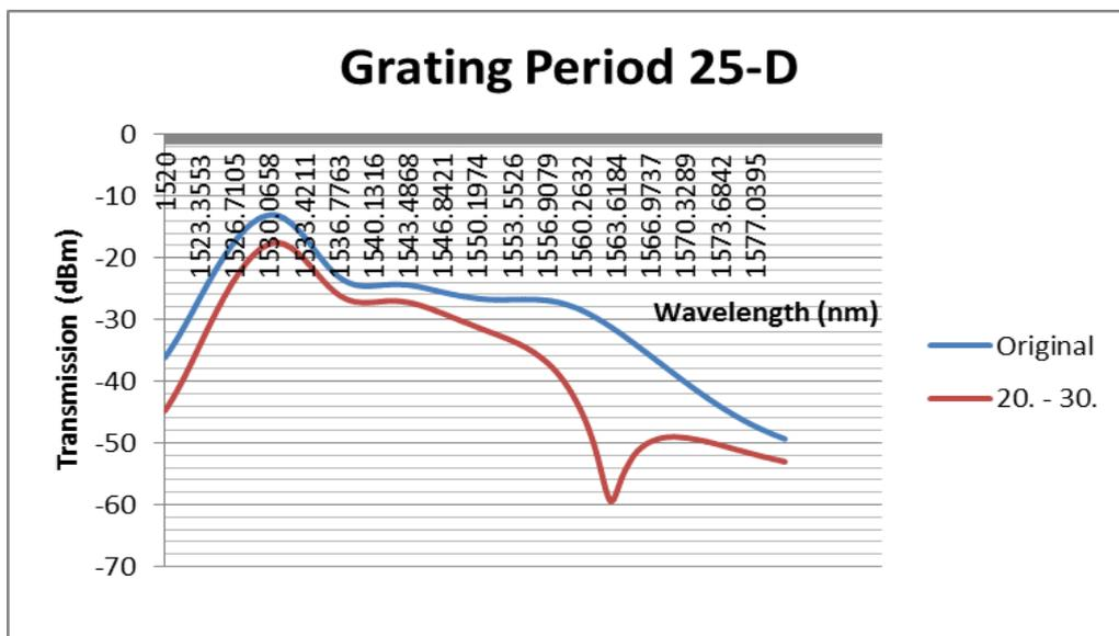
Figure 4.1-5: Comparison between the original points with the notch
