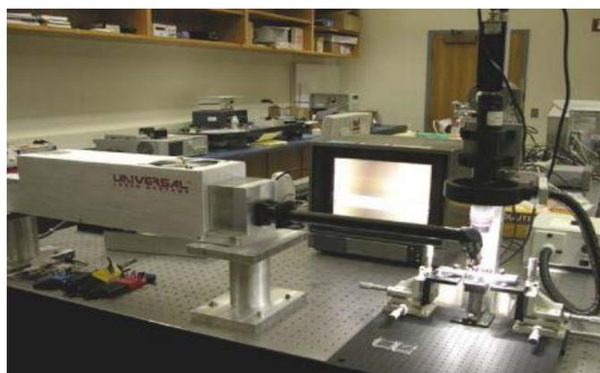
Figure 2.2-2: Photograph of LPFG fabrication system
