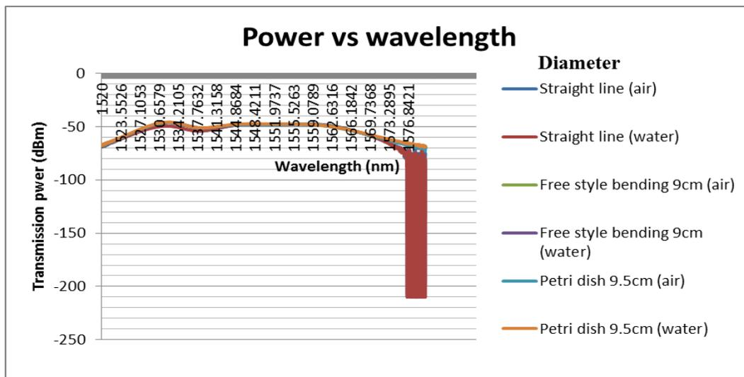
Figure 4.5-1: Fiber with 33 grating period with 22g test under air and water condition with different bending structures
