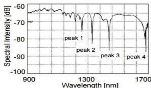
Figure 2.4-2: Transmission spectrum of an LPFG with a grating period of 212  $\mu\text{m}$  and a grating length of 30 mm, exposure time was 18 h. (Mizunami, 2014)
