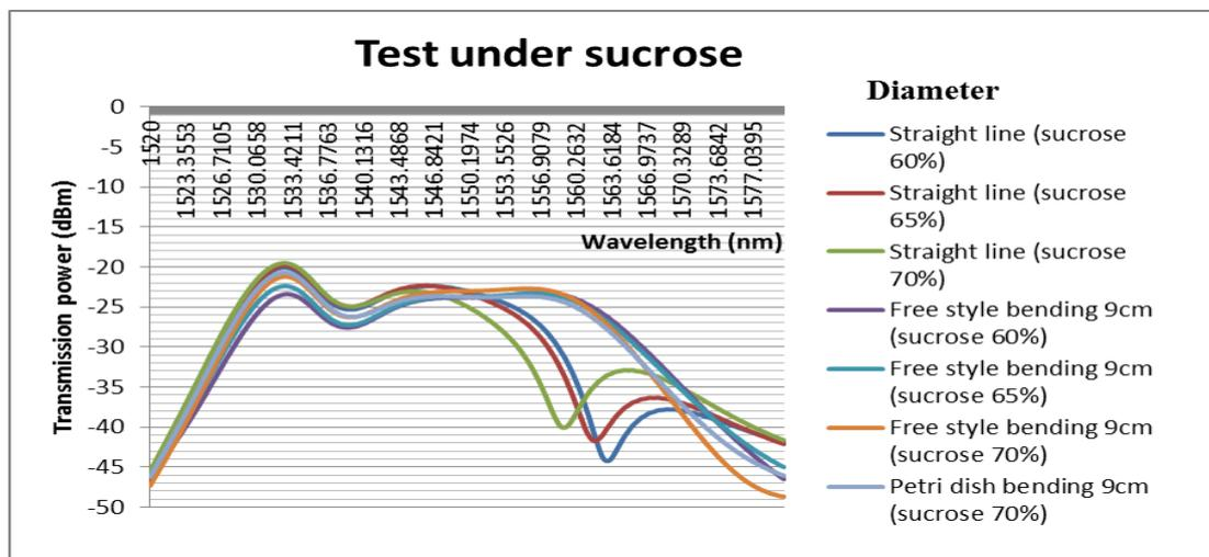
Figure 4.3-4: The weight with 14g and 18 number of grating period fiber was tested under the sucrose condition with different structures
