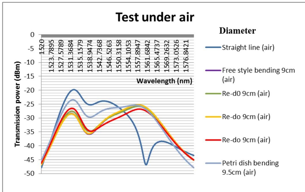
Figure 4.3-13: The weight with 14g and 40 number of grating period fiber was tested under air condition with different bending structures
