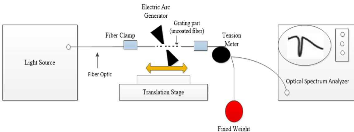
Figure 2.1-1: Experimental setup used for LPFG by the micro-taper method
