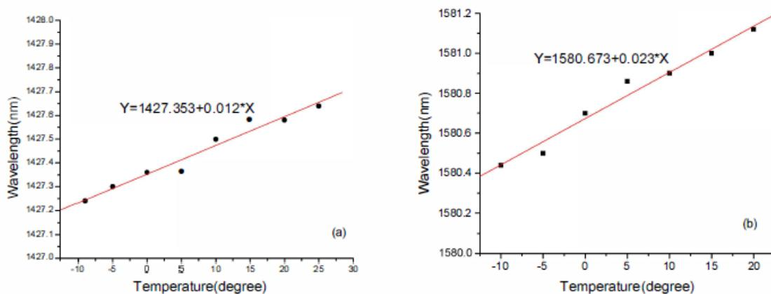
Figure 2.3-3: Temperature dependence of dip wavelength shift of LPFG in air. (a). The temperature sensitivity of LPFG without encapsulation was measured to be  $12\text{ pm}/^{\circ}\text{C}$ . (b). The temperature sensitivity of LPFG encapsulated was measured to be  $23\text{ pm}/^{\circ}\text{C}$
