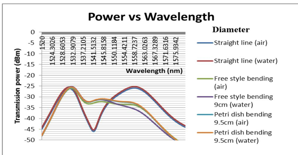
Figure 4.6-1: Fiber with 25 grating period with 22g test under air and water condition with different bending structures
