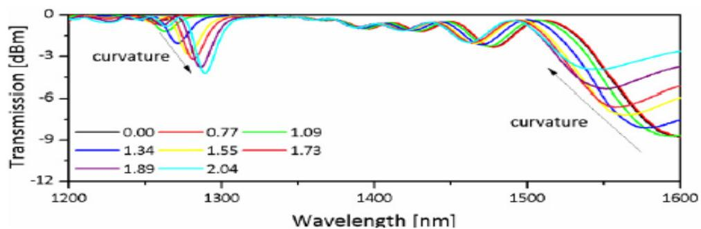
Figure 2.6-1: Effect of bending given in m-1 LPG transmission spectrum (M. Szymańska, 2014)
