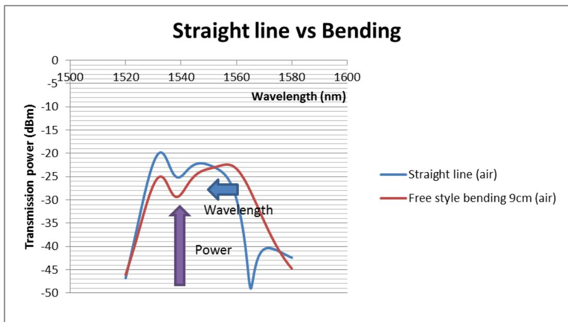
Figure 4.3-2: Comparison between straight with bending method. Power was drop from -49.037dBm to -29.352dbm. Wavelength was shift 26.605nm to left side
