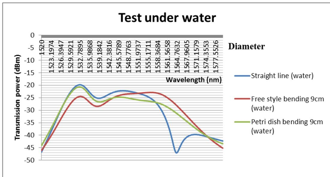
Figure 4.3-3: The weight with 14g and 18 number of grating period fiber was tested under the water condition with different structures
