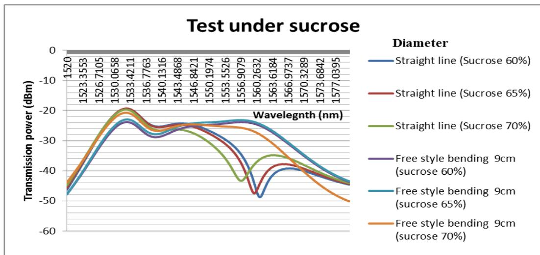
Figure 4.3-10: The fiber with 29 number of grating period was tested under sucrose condition
