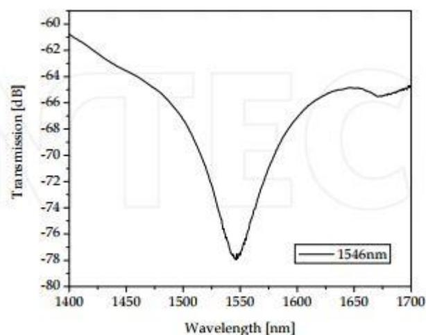
Figure 2.1-5: Loss band of a fattened long period grating near 1550 nm
