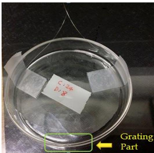
Bending test in Petri Dish
