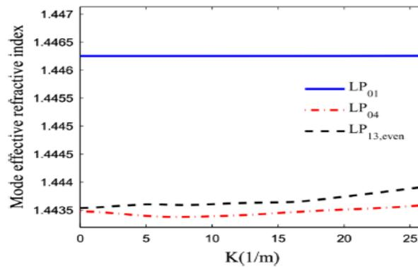
Figure 2.5-2: At the different bending curvatures, to obtain the effective refractive indexes of LP<sub>01</sub>, LP<sub>04</sub>, and LP<sub>13, even</sub> modes
