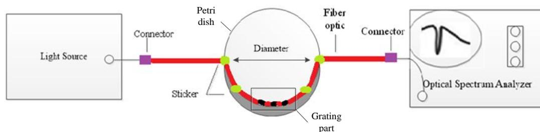
Figure 3.2-2: Experimental Setup for bending structure in petri dish
