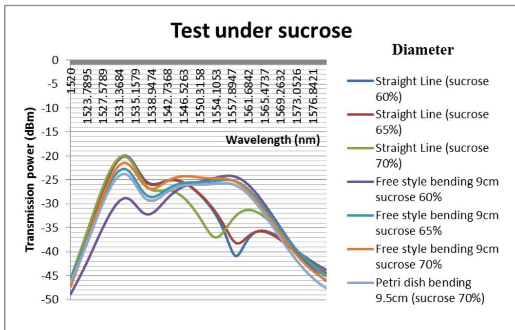
Figure 4.3-16: The weight with 14g and 40 number of grating period fiber was tested under sucrose condition with different bending structures
