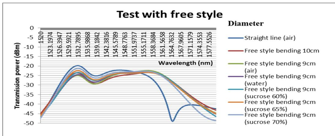
Figure 4.3-6: The weight with 14g and 18 number of grating period fiber was tested with free style in plastic sheet
