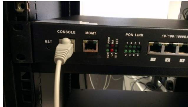
Figure A.4: Console port connection
