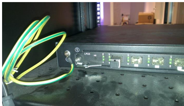
Figure A.3: Ground connection of OLT
