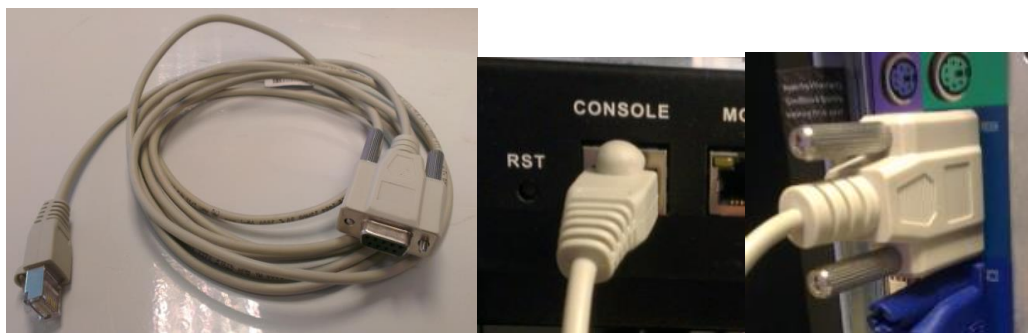
Figure 4.3: RJ45 to DB9 Cable and connection
