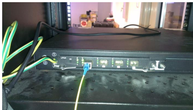
Figure A.7: Backward connection of OLT
