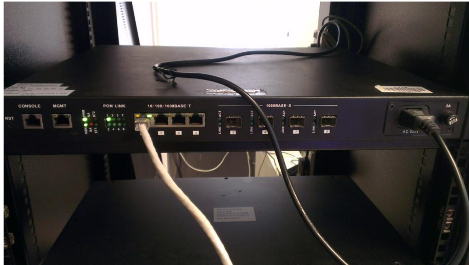
Figure A.18: Unplug the console port and connect the uplink port using Ethernet cable
