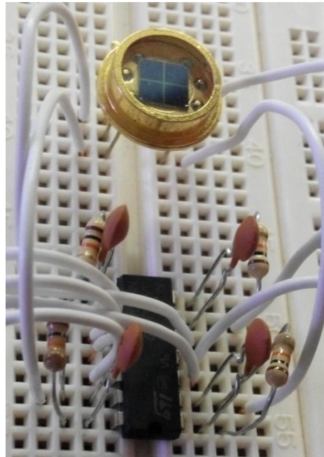
Figure 21: 4 internal op-amp for 4 pins of photodiode
