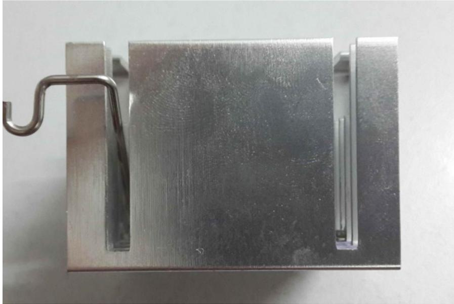
**Fig.3.2:** Side view of Heat sink
