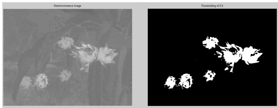
Figure 3.4: Convert grayscale image into binary image by thresholding of 0.6.
