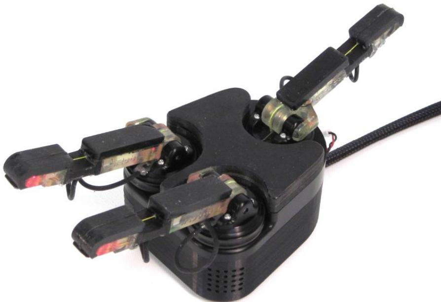
**Figure 2-2-1: Structure of three fingers robotic hand**
