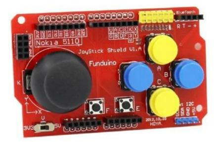
Figure 3-6-1: Actual view of Arduino joystick shield module
