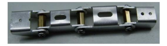
Figure 3-3-2: Structure of robotic hand's finger top view
