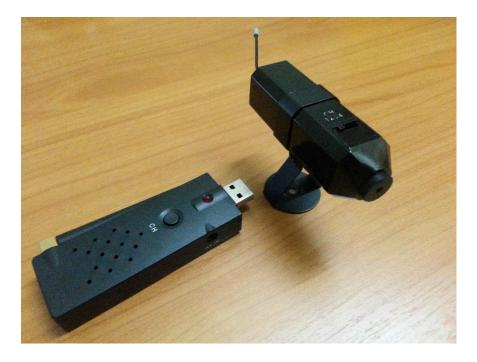
Figure 6-1-1: Wireless camera and USB receiver
