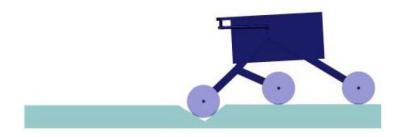
Figure 2-1-6: Six-wheel mobile robot traversing over a ditch
