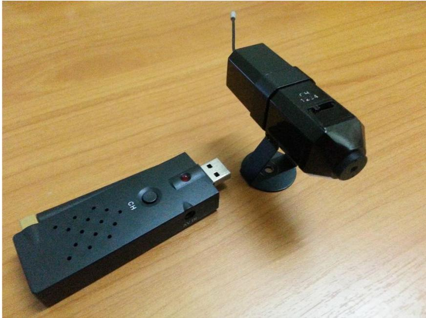
**Figure 6-1-1: Wireless camera and USB receiver**
