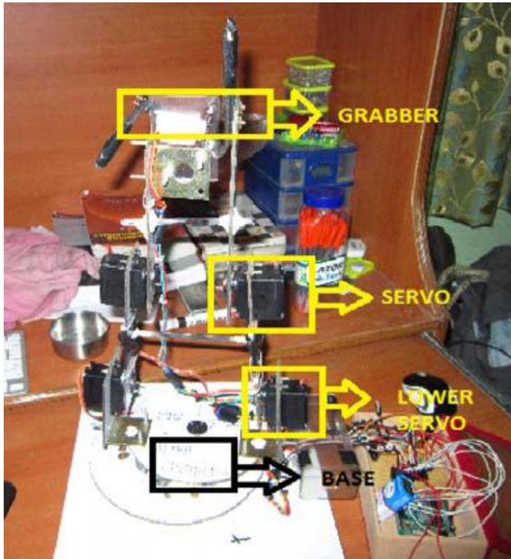
**Figure 2-4-2: Robotic arm servo alignment front view**
