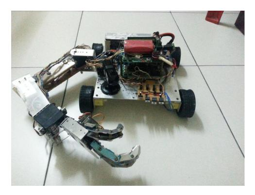
Figure 5-4-1: Mobile robot unit front view
