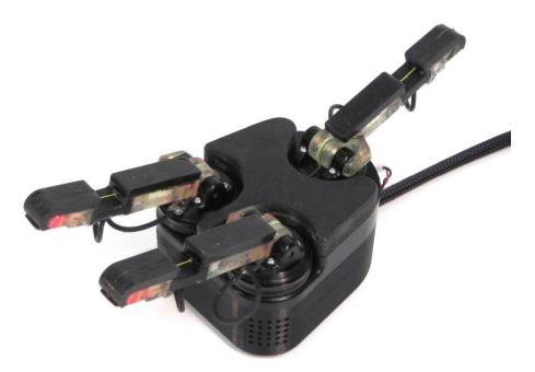
Figure 2-2-1: Structure of three fingers robotic hand
