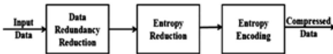
Figure 2-4: Basic model of compression system (Ruchika, Singh & Singh 2012).
