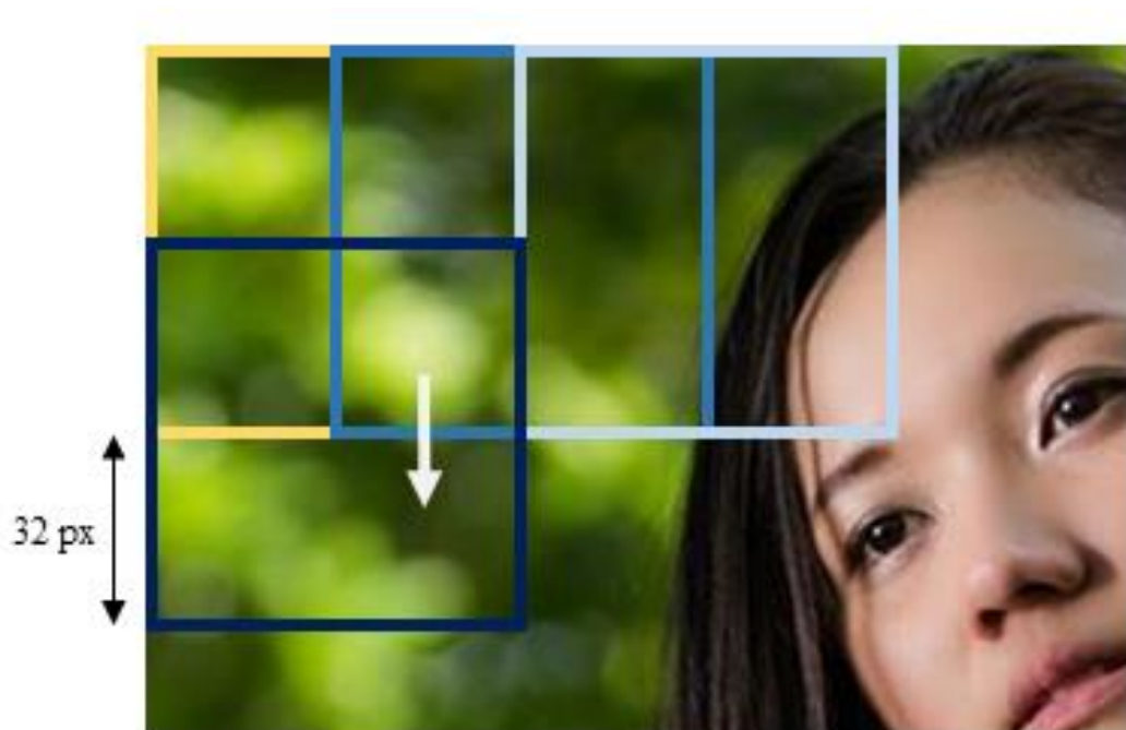
Figure 3-13: Kernel will be moved to lower position after reaching right end of photo image.
