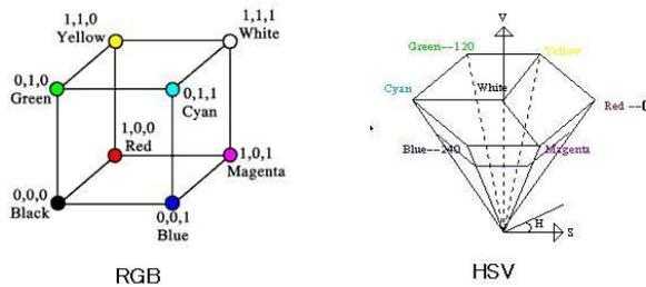
**Figure 3:** RGB and HSV colour space representation
