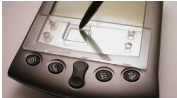
Figure 6: Transparent plastic cover used for EdgeWrite text entry.
