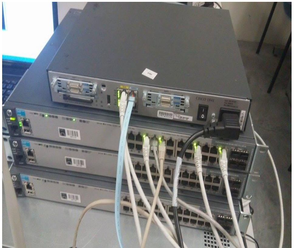
Figure 5.1.2.1: The device on the second row with light on is HP Switch 2920-24G while the device at the top is Cisco Router 1841.
