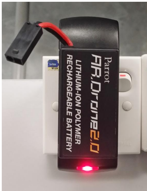
Figure 5-1-2: Recharging battery process in progress – red color LED
