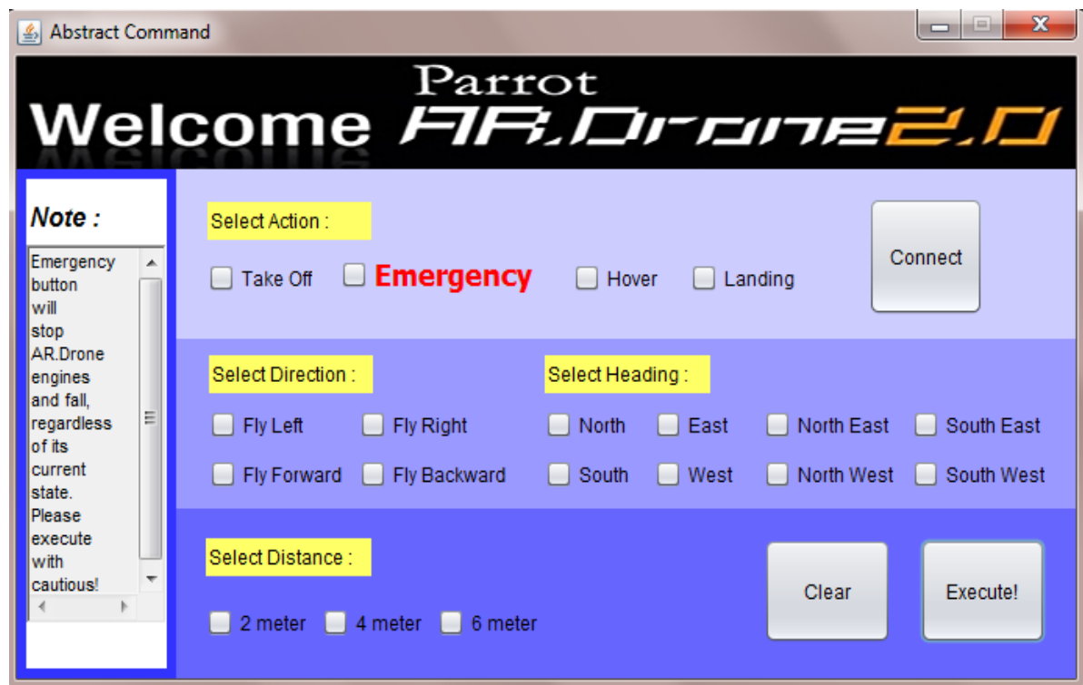
Figure 5-4-44: Press “Clear” button to uncheck all abstract command checkboxes and delete the previous abstract command
