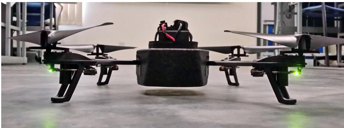
Figure 5-1-5: 4 motor LED green lights indicates startup is okay
