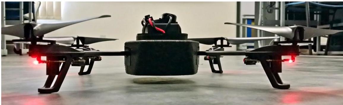
Figure 5-1-6: 4 motor LEDs shows red lights
