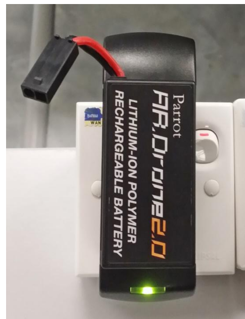
Figure 5-1-3: Recharging battery done – light green color LED
