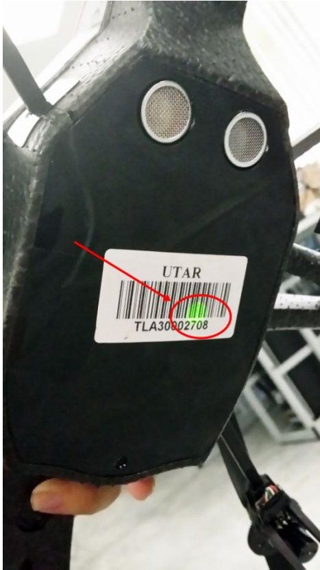
Figure 5-1-8: System LED shows green color
