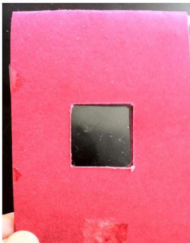
**Figure 3.6: Photograph of XNBR Latex Thin Film.**
