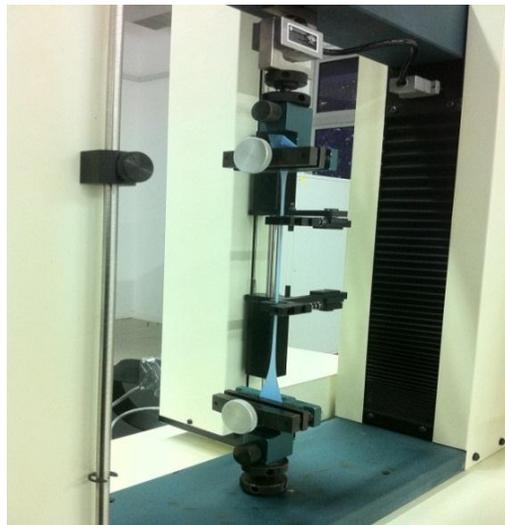
**Figure 3.2: Photograph of tensile strength measurement.**
