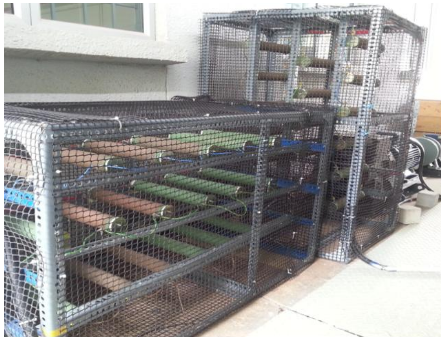
Figure 3.11 Load emulators installed in the laboratory
