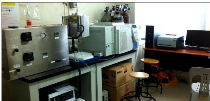
**Figure 3.9: Fixed-bed microreactor with on-line Thermo Scientific TRACE GC**
