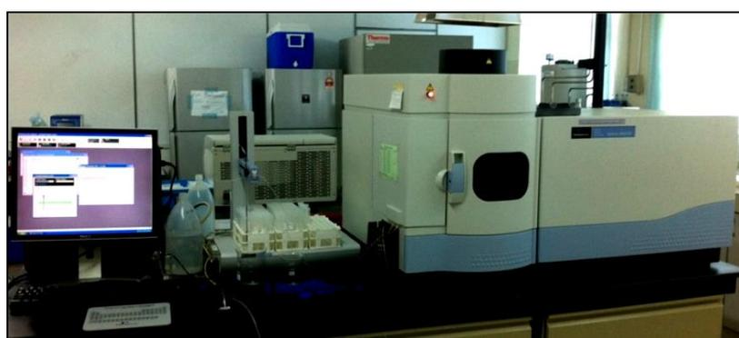
**Figure 3.7: Perkin Elmer Optima 2000 DV optical emission spectrometer**
