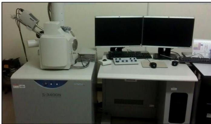
**Figure 3.5: Hitachi S-3400N electron microscope coupled with EDAX software**
