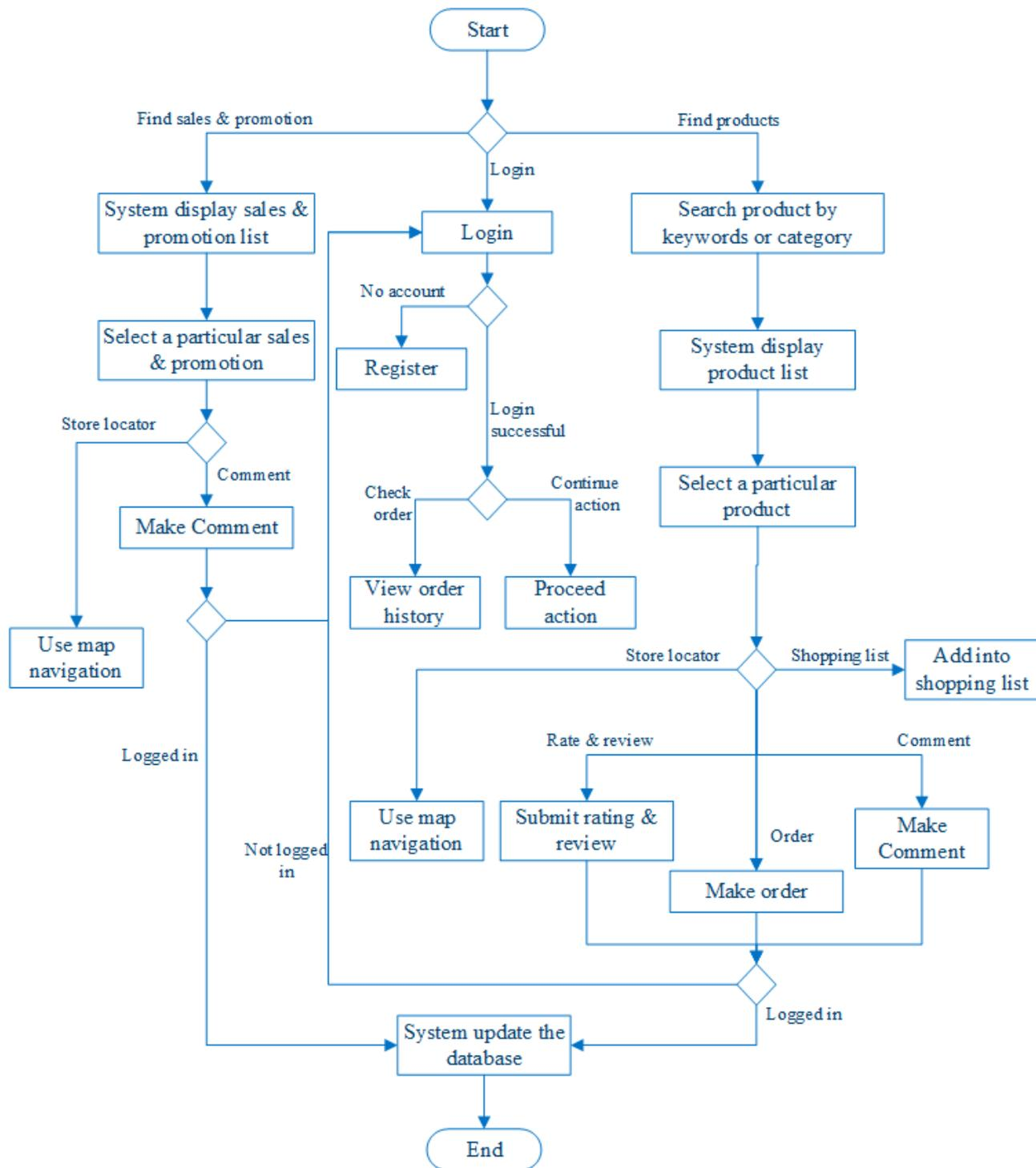
Figure 3-2 Shopper's side system flowchart
