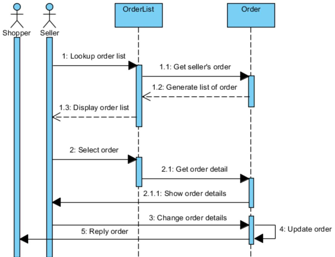
Figure 3-14 Manage order sequence diagram
