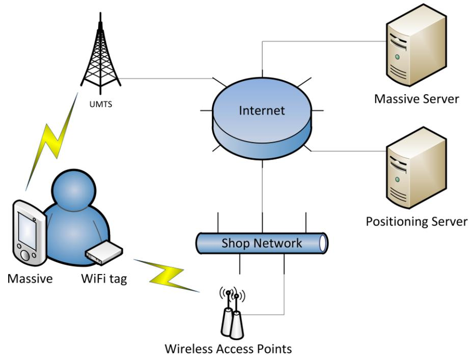
Figure 2-2 Ma\$\$ive Architecture Diagram (Sourav Bhattacharya, 2012)
