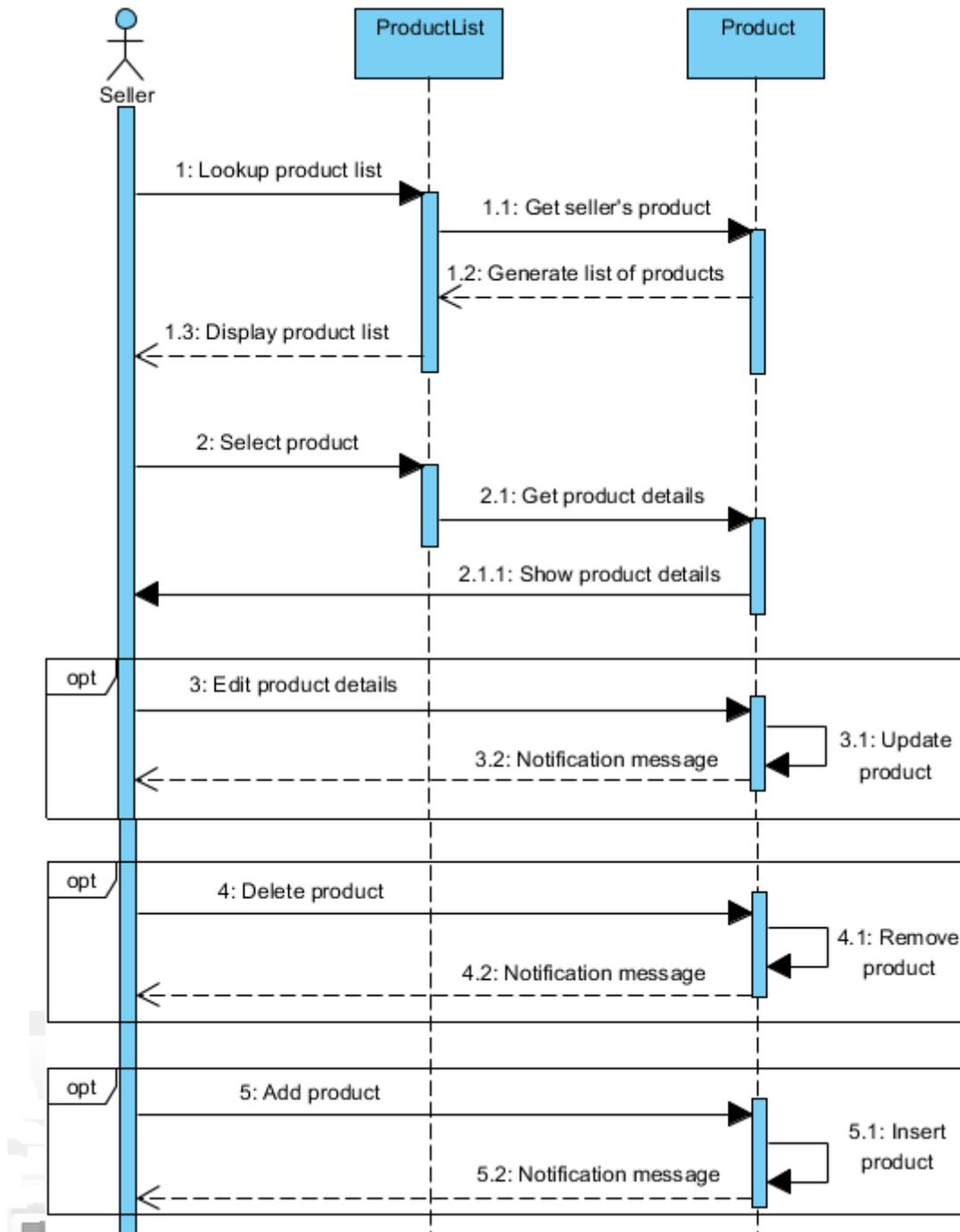
Figure 3-15 Manage product sequence diagram
