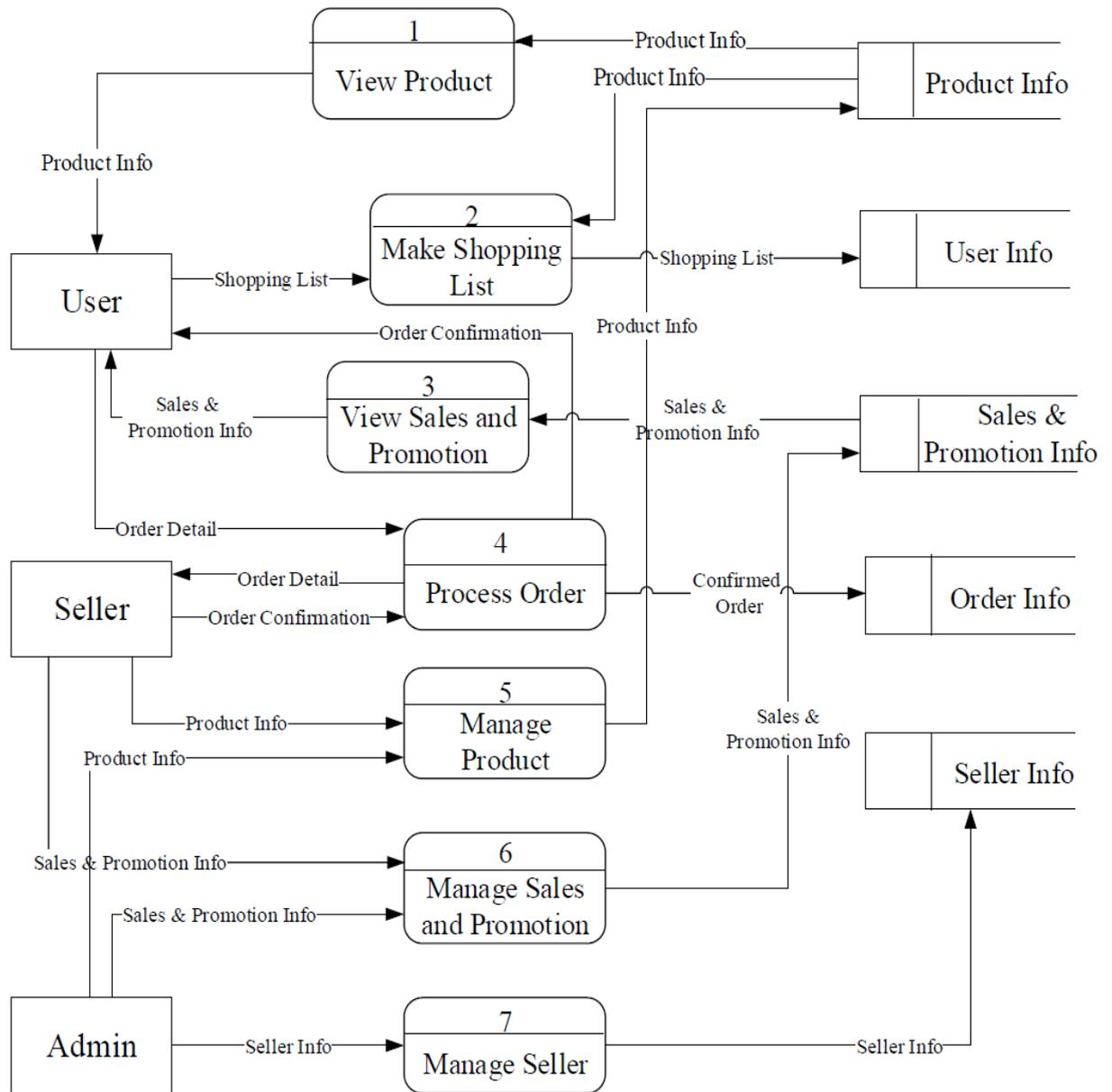
Figure 3-19 Level-1 Data Flow Diagram
