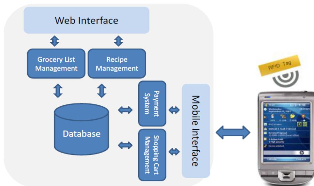
Figure 2-5 Architecture and Main Components Diagram (Lilac A. E. Al-Safadi, 2010)
