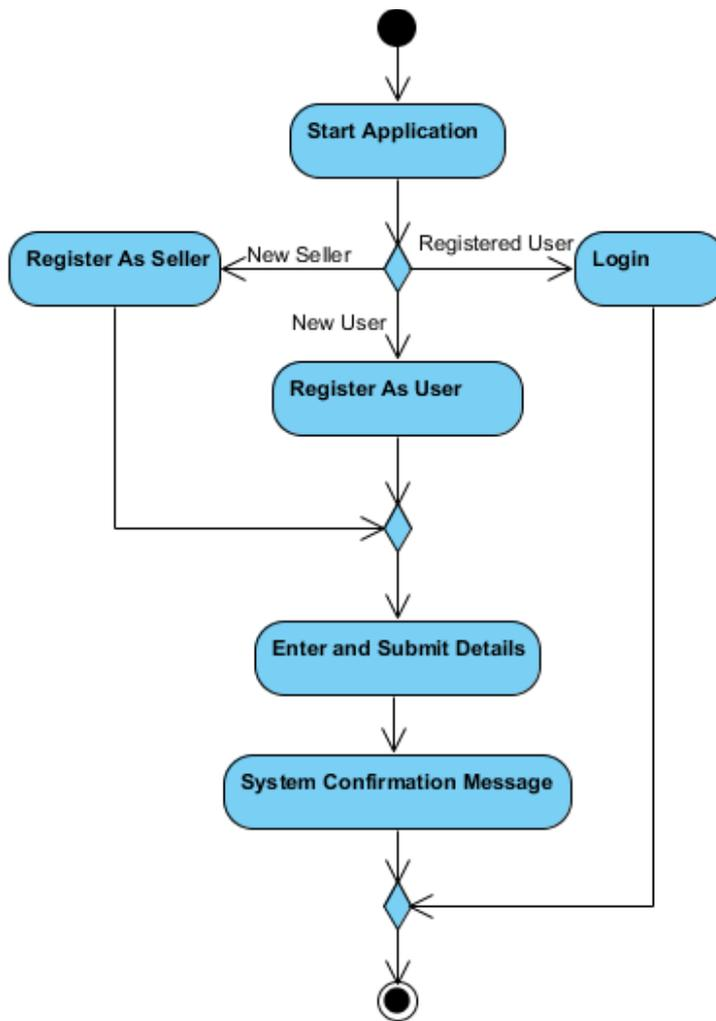
Figure 3-5 Register Activity Diagram
