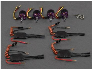
Fig. 4.3: Rotors and ESCs (HobbyKing.com 2014)
