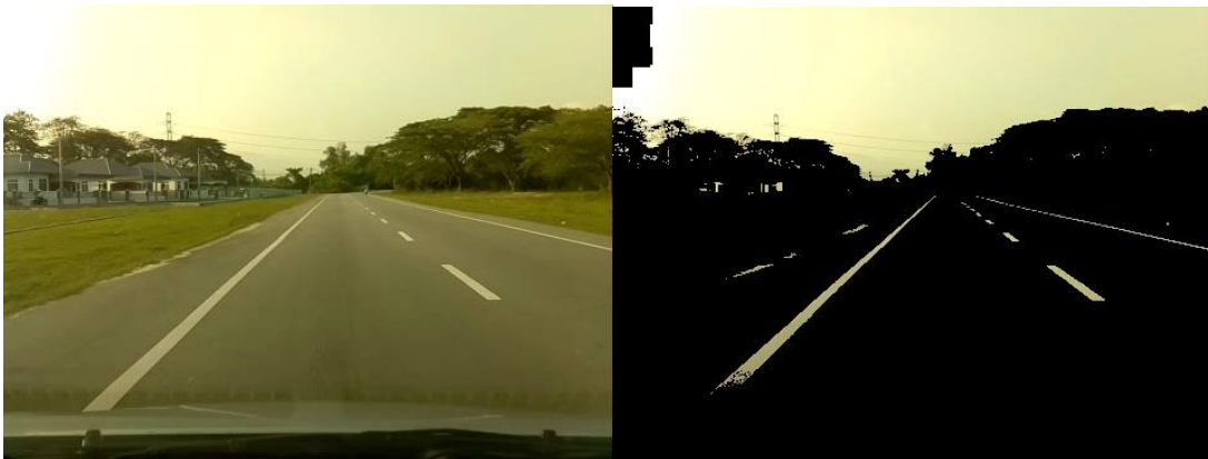
Figure 28 Input image and filtered image
