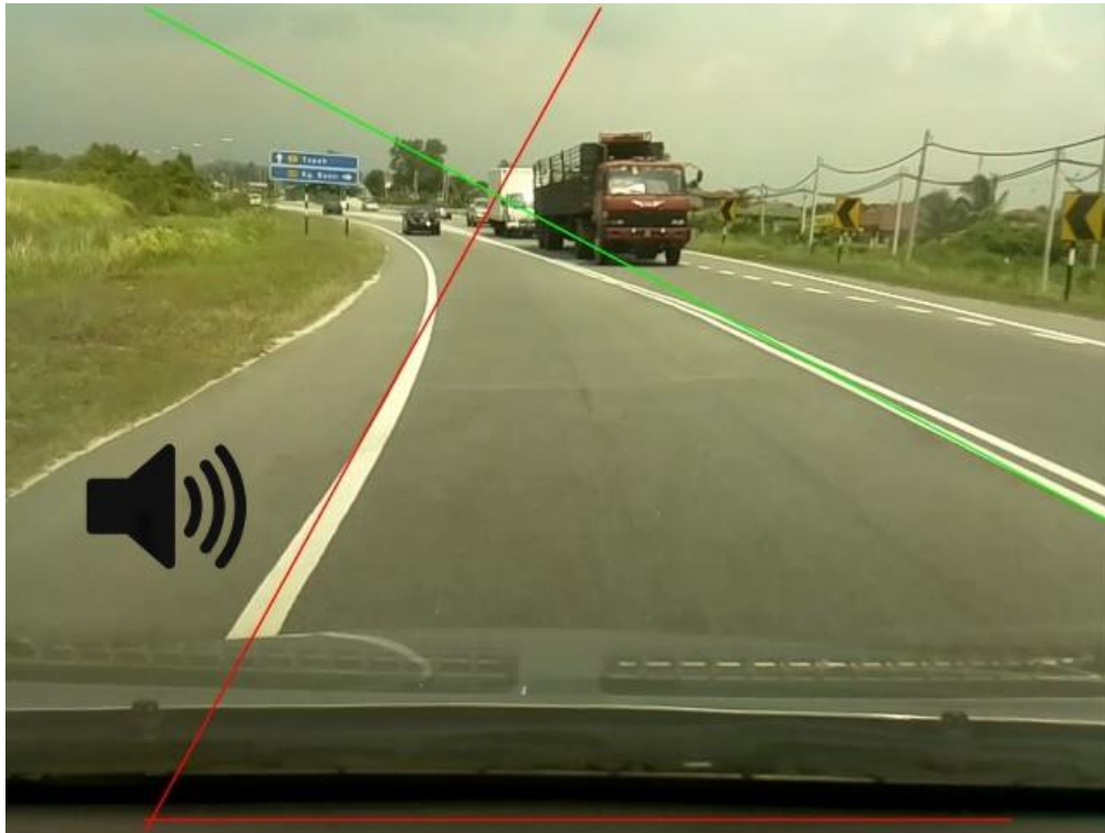
Figure 2 Simple illustration of how LDWS work.
