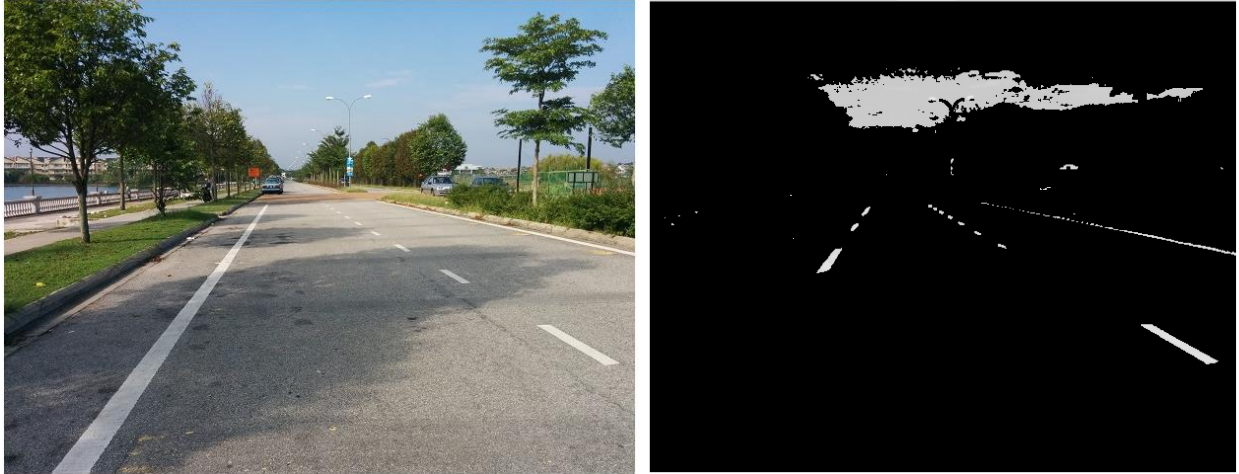
Figure 25 Input Image and standard thresholding output
