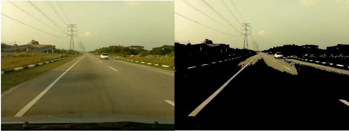
Figure 29 Input image and result image of imperfect filter
