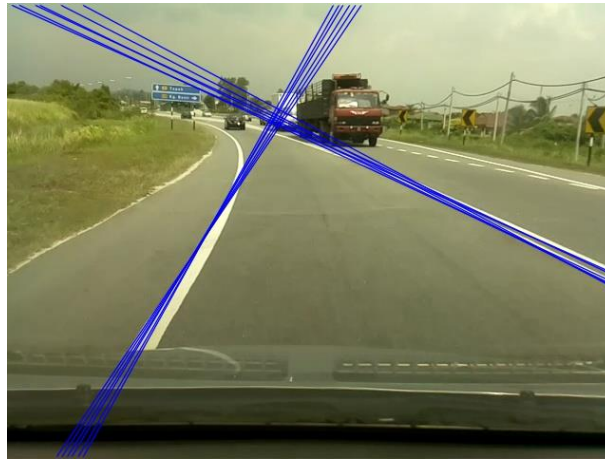
Figure 20 Line detected in Hough Line Transform
