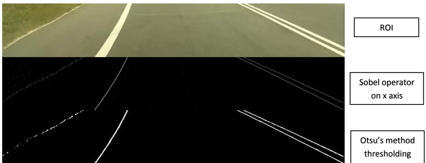
Figure 19 Output of Sobel operator and Otsu thresholding on ROI image
