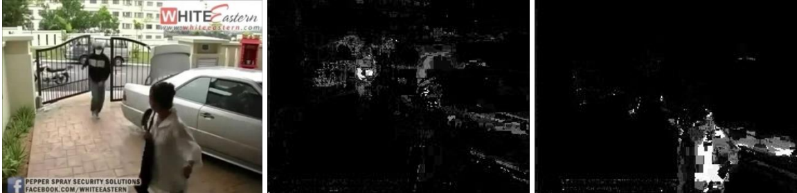
Figure 4.19 Image with original frame (left), back projection of the intruders' tracker (center), and back projection of the owner's tracker (right)
