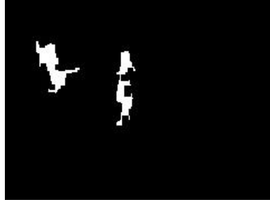
Figure 4.15 Result of connected components analysis and blob filtering
