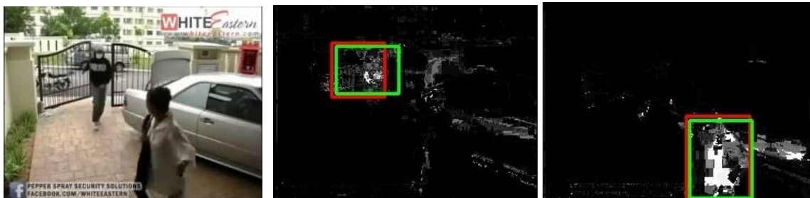
Figure 4.20 Image with original frame (left), CAMSHIFT of the intruders' tracker (center), and CAMSHIFT of the owner's tracker (right)
