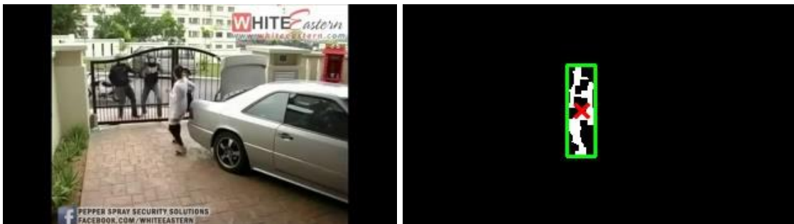
Figure 4.18 Images with original frame (left) and information obtain from the object's blob (right)
