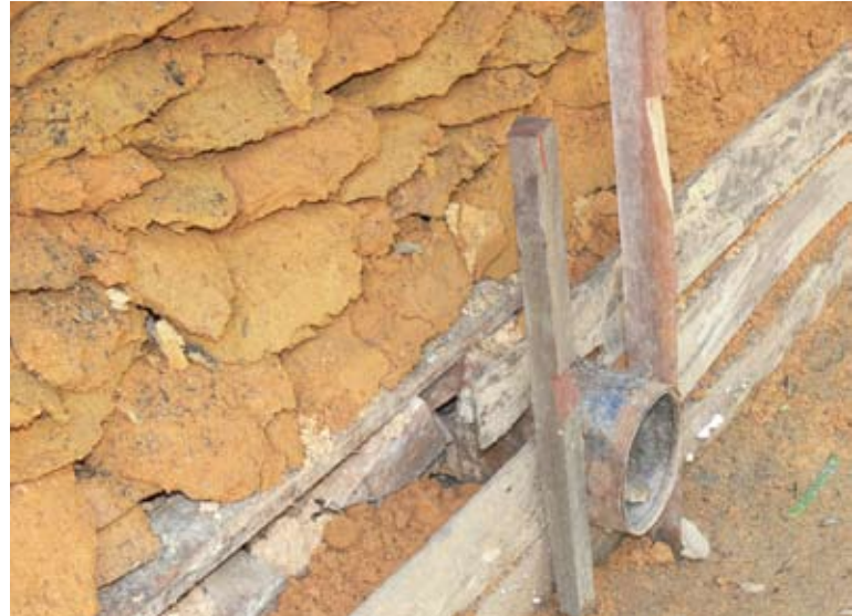
Blocks of earth stacked on top of waste wood in a pyre
