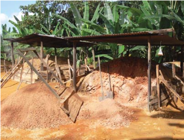
After the burn, the burnt earth is sieved
