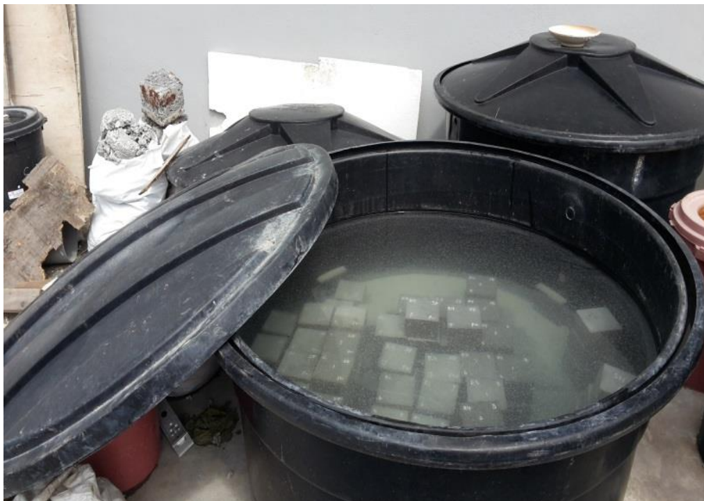
Figure 3.9 Mortar Curing Process
