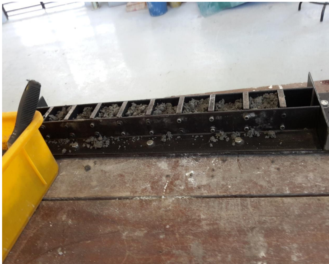
Figure 3.8 Mould Use to Cast 50 mm x 50 mm x 50 mm Mortar
