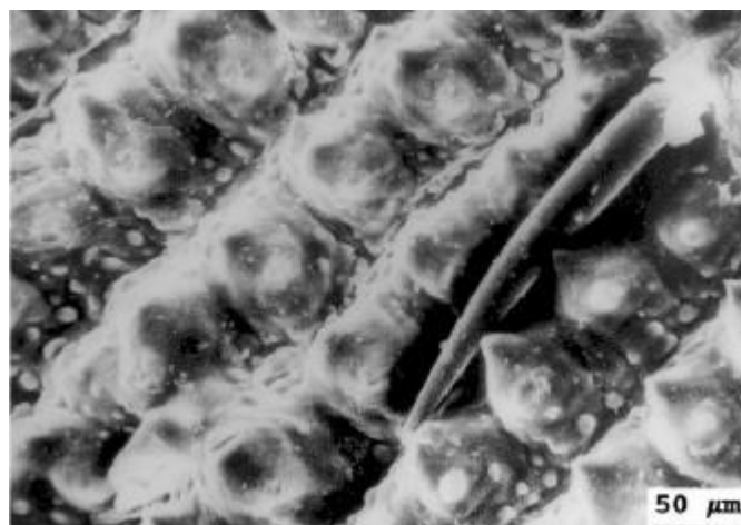
Figure 2.5 SEM Micrographs of Outer Epidermis of RH Treated by 3 N HCl (Krishnarao, Subrahmanyam and Jagadish Kumar, 2001)
