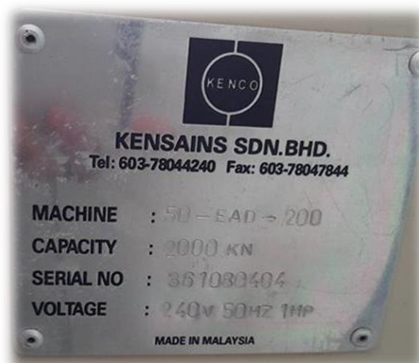
Figure 3.11: Specification of Kenco Compressive Strength Testing Machine
