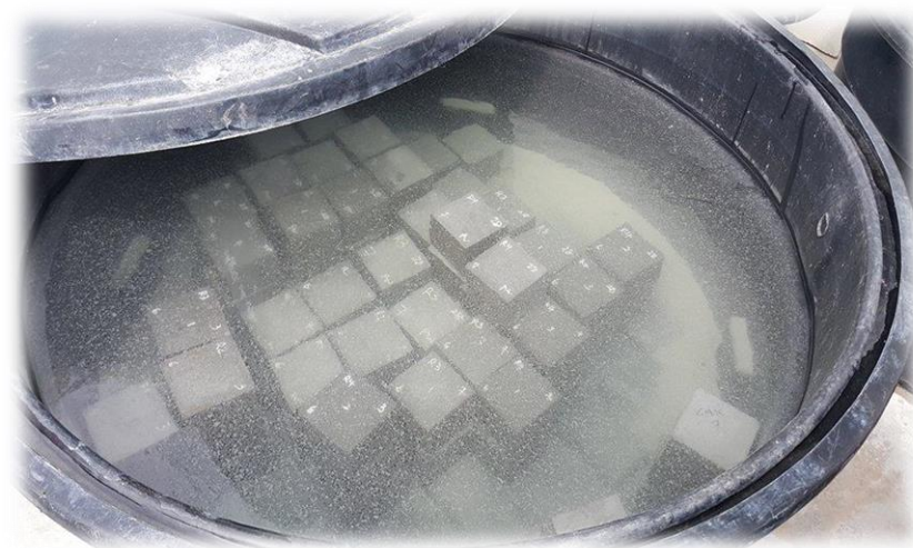
Figure 3.8: Water Curing of Concrete Specimens
