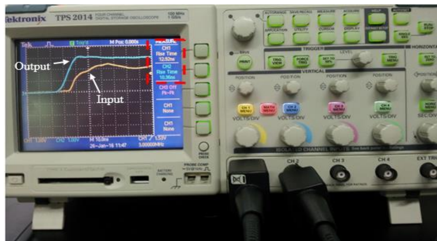
Figure 4.2: Rise time measurement of output buffer
