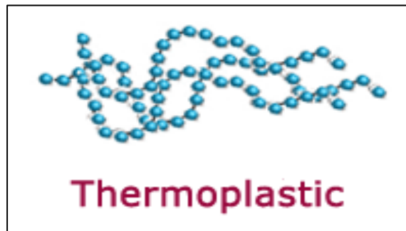
Figure 2.6: Linkage of Polymer in Thermoplastic (Adhesiveandglue.com, 2015)
