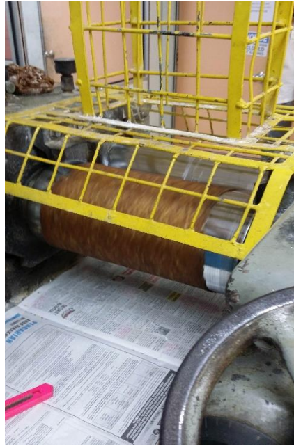
Figure 3.7: Natural rubber compounding in two roll mills
