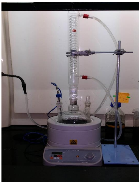
Figure 3.4: Solution heated in heating mantle with stirrer at 100 °C under a water-cooled condenser for 24 hour
