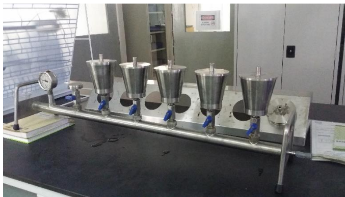
Figure 3.5: Product cooled, filtered and washed with copious amount of deionized water
