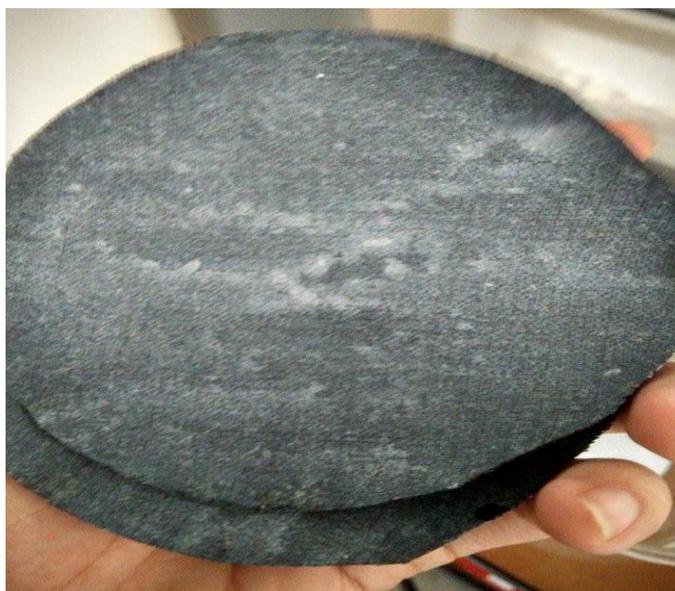
**Figure 3.1: The air facing cathode layer.**
