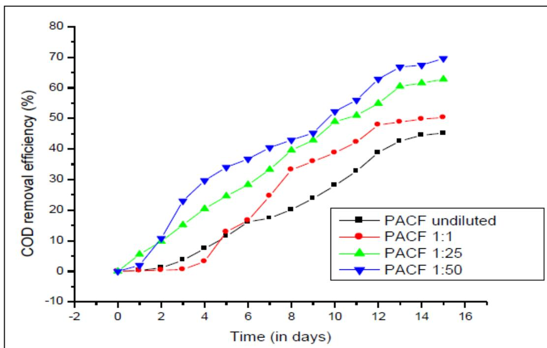
**Figure 2.5: COD removal efficiency of PACF MFC at different dilutions of raw POME with time (Baranitharan, Maksudur and Prasad, 2013).**
