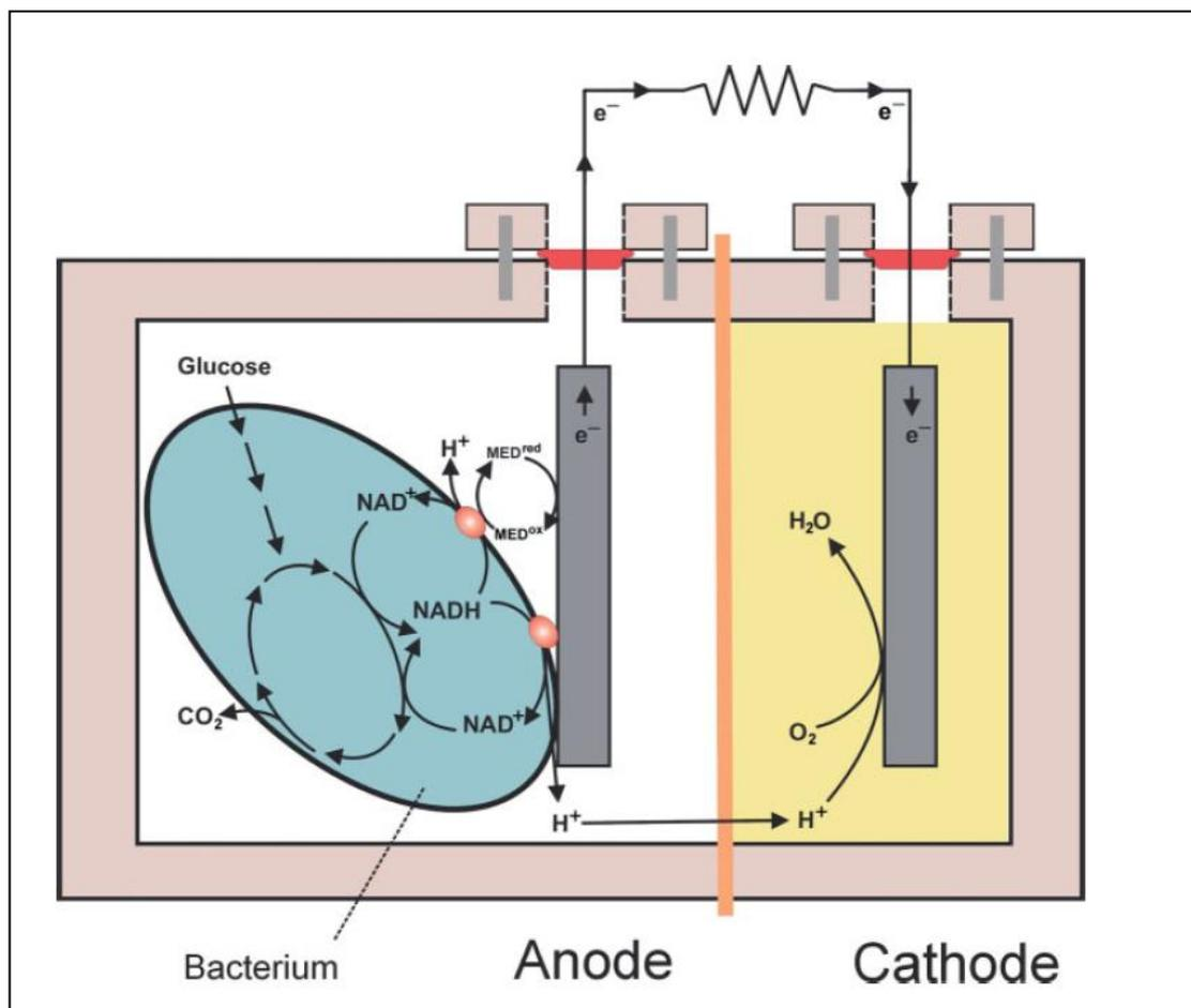
**Figure 2.2: Graphical Microbial Fuel Cell (Pham et al., 2006).**
