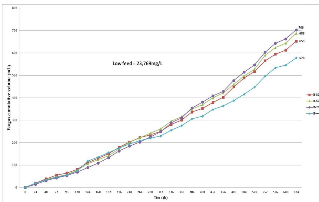
**Figure 4.9: Biogas cumulative volumes over 624 hours for four low concentration feed MFCs.**
