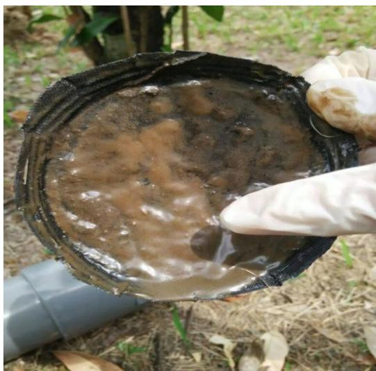
Figure B2: Deposition layer found on the air cathode surface of MFC.
