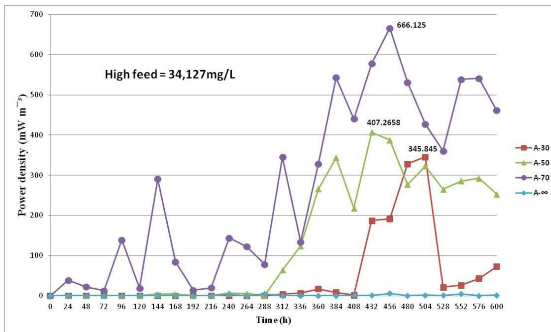
**Figure 4.3: Power density over 600 hours for four high concentration feed MFCs with different SRTs.**
