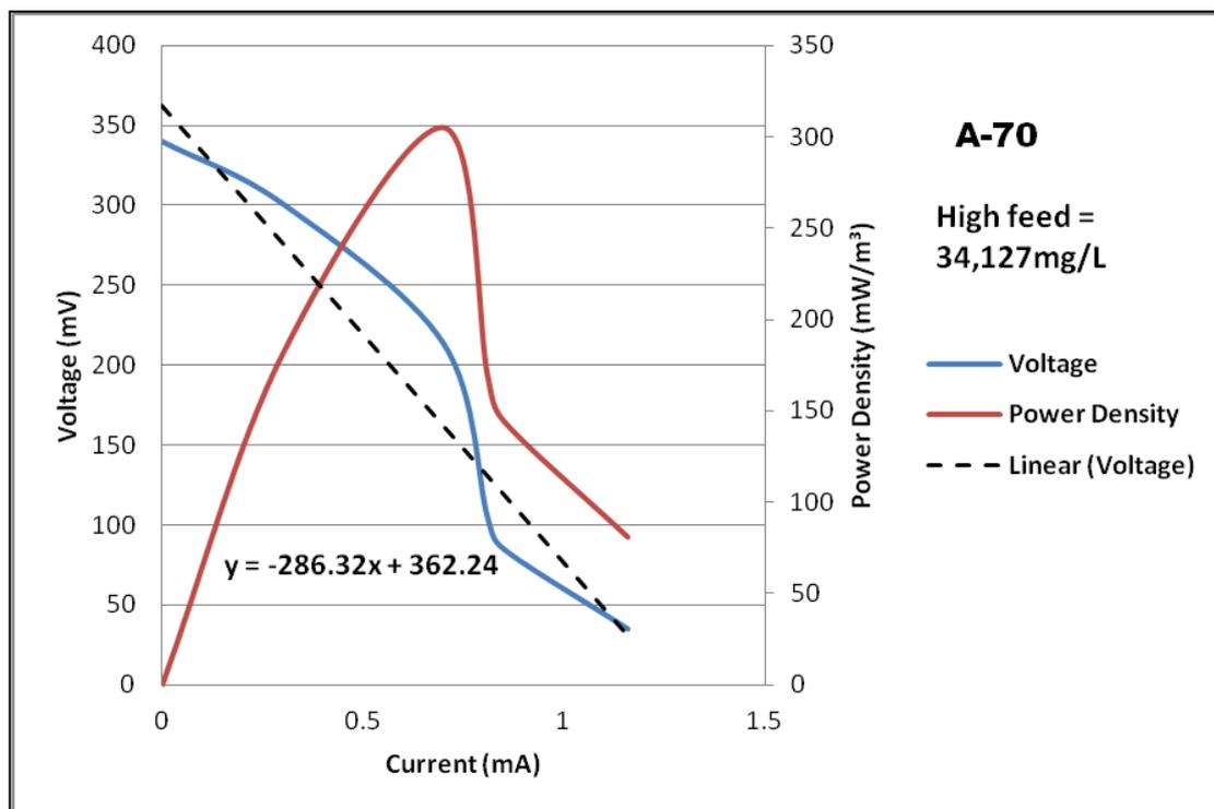
Figure 4.7: Polarization curve for SRT 70 days and high concentration feed MFC.
