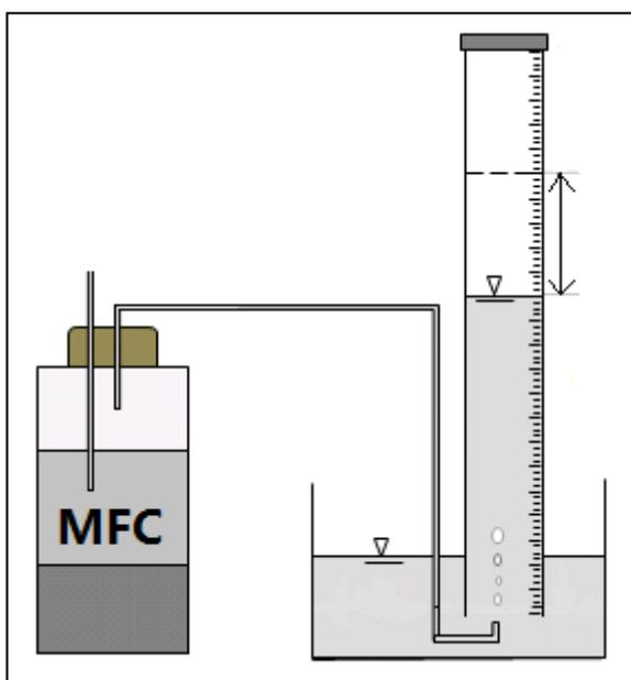
**Figure 3.4: Schematic diagram of biogas collection using water displacement method.**
