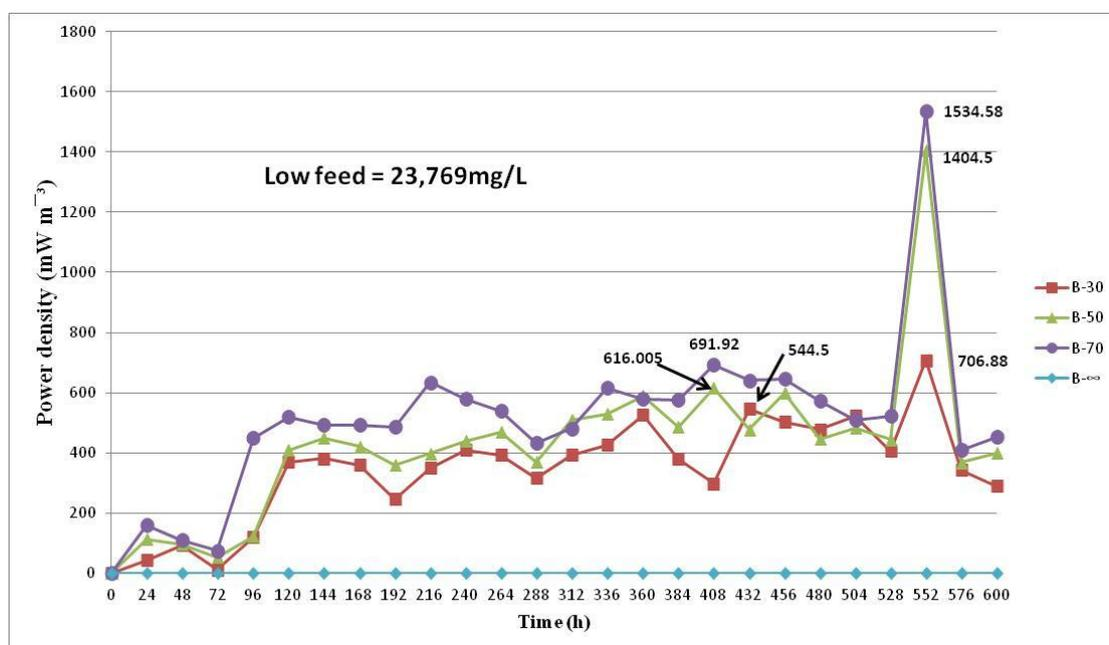
**Figure 4.5: Power density over 600 hours for four low concentration feed MFCs with different SRTs.**
