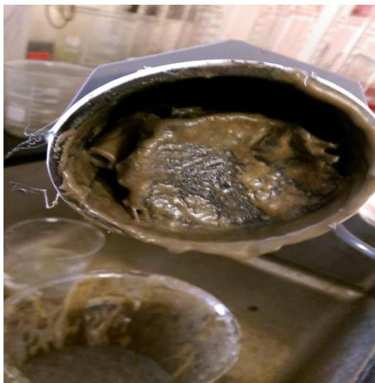
Figure B1: Deposition layer found on the anode surface of MFC.
