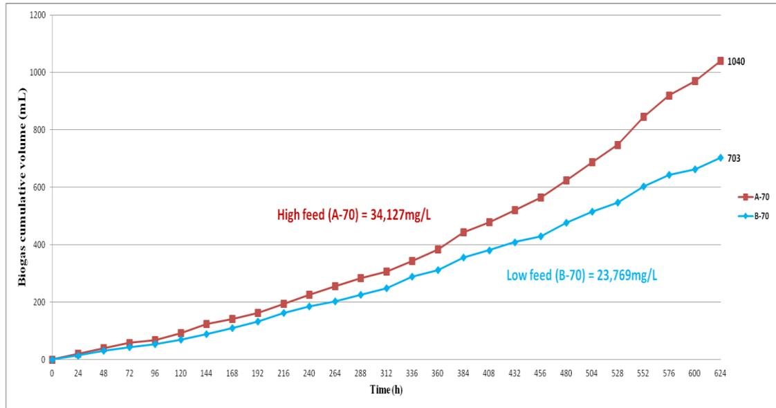
**Figure 4.10: Comparison of biogas cumulative volumes over 624 hours for two different concentration feed MFCs at SRT 70.**
