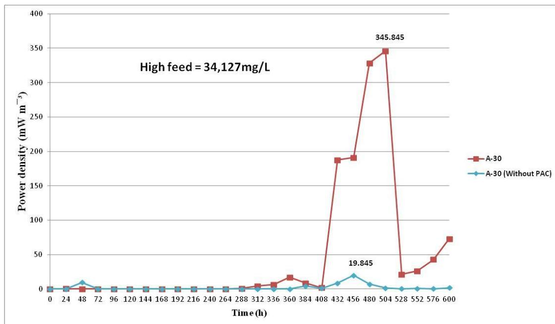
**Figure 4.1: Power density over 600 hours for MFCs added with and without PAC.**
