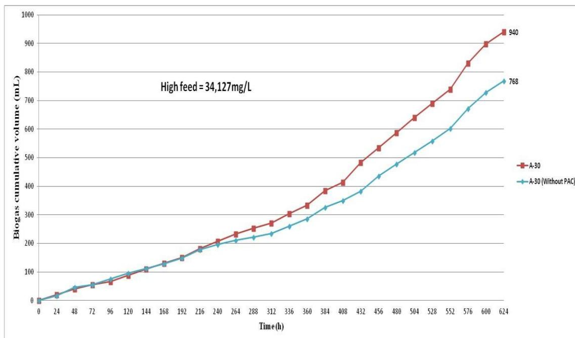
**Figure 4.2: Biogas cumulative volumes over 624 hours for MFCs added with and without PAC.**
