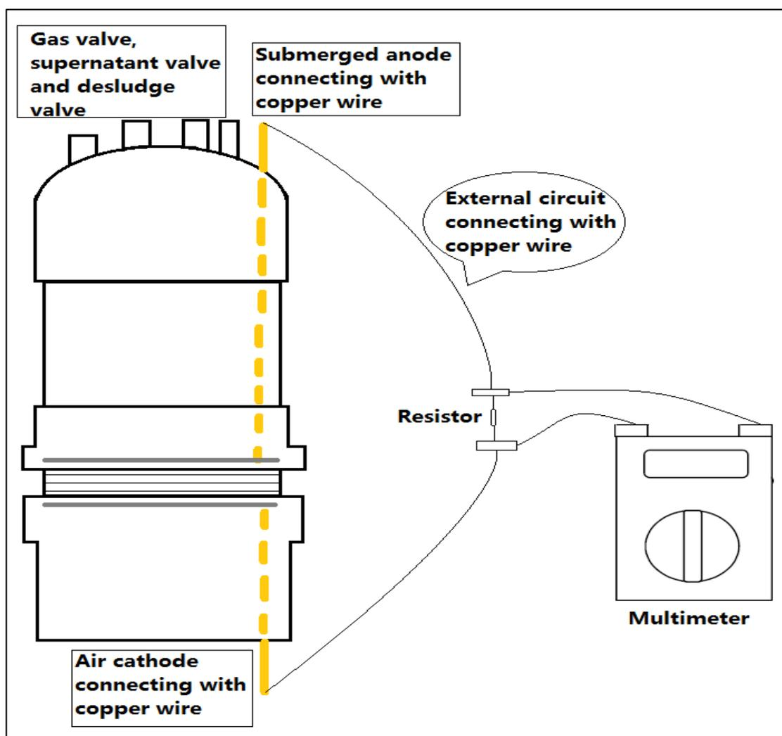
**Figure 3.3: The schematic diagram of MFC.**
