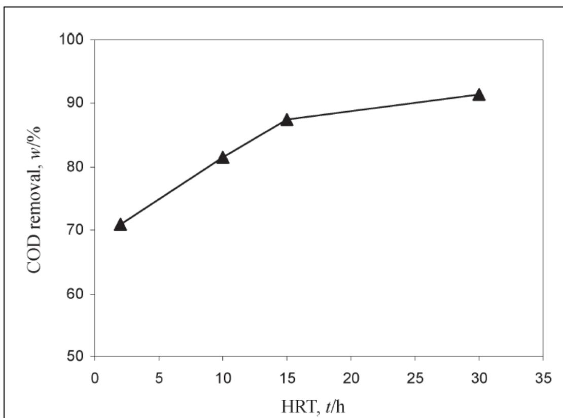
**Figure 2.4: Effect of HRT on different parameter removal rate.**
