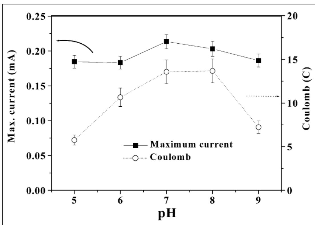
Figure 2.3: Effects of pH on the performance of MFC (Gil et al., 2003).
