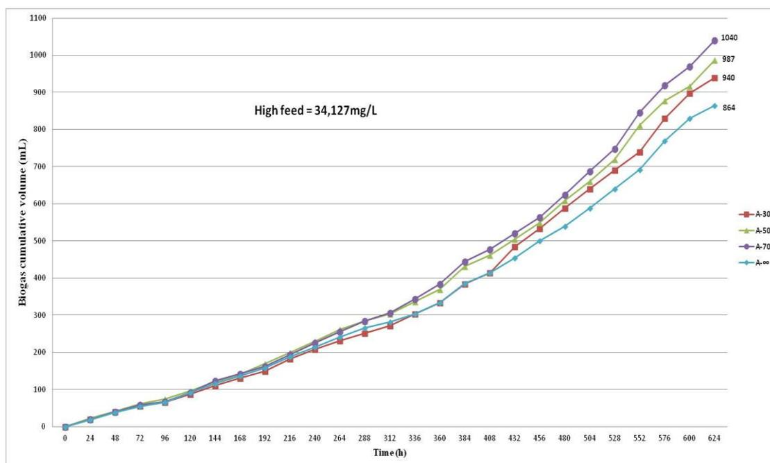
**Figure 4.4: Biogas cumulative volumes over 624 hours for four high concentration feed MFCs with different SRTs.**
