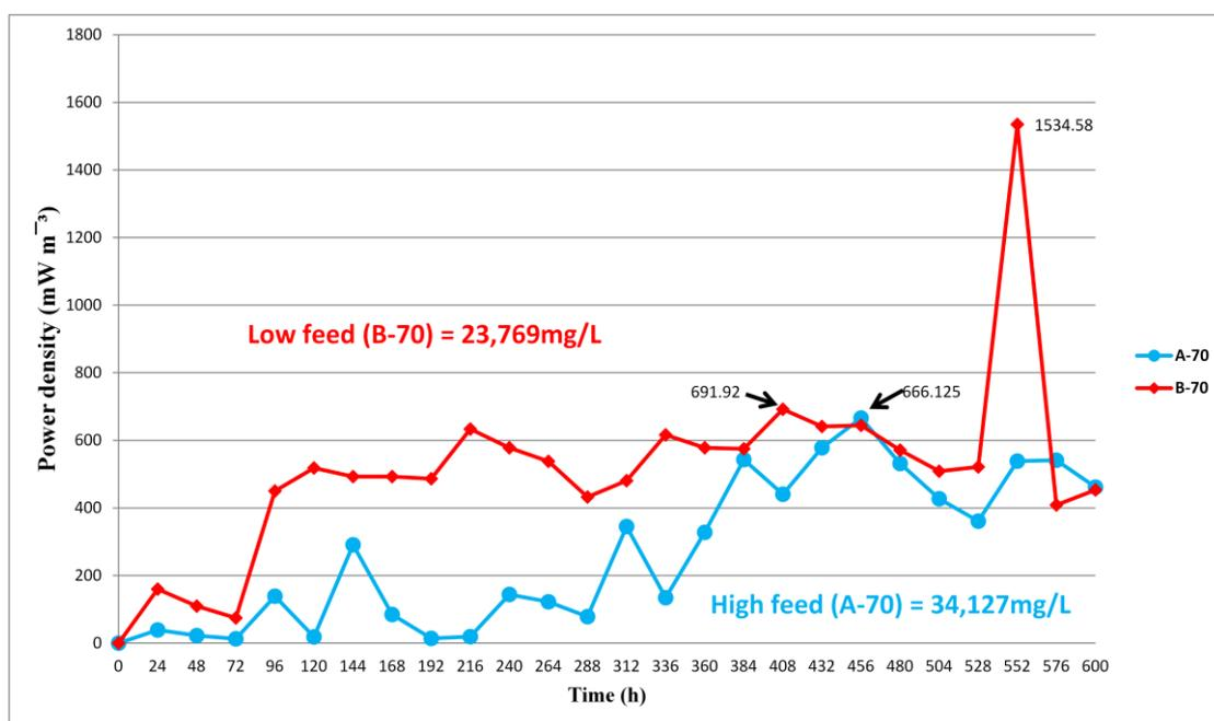
**Figure 4.6: Comparison of power density over 600 hours for two different concentration feed MFCs at SRT 70.**
