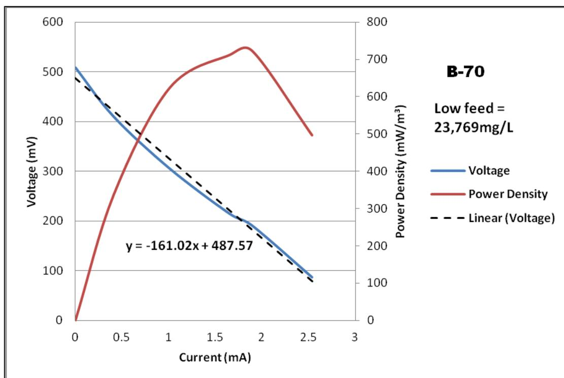
Figure 4.8: Polarization curve for SRT 70 days and low concentration feed MFC.
