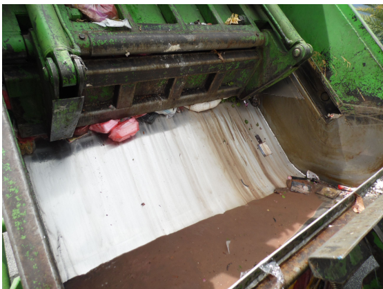
Leachate flowing out from the waste
