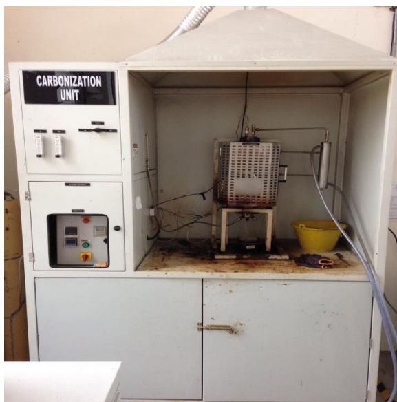
Figure 3.2: Carbonization Unit Used to Prepare Palm Oil Sludge Bio-Char Samples
