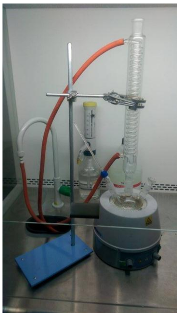
Dope preparation equipment setup
