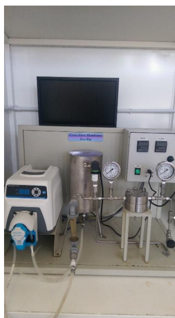
Cross Flow Filtration System
