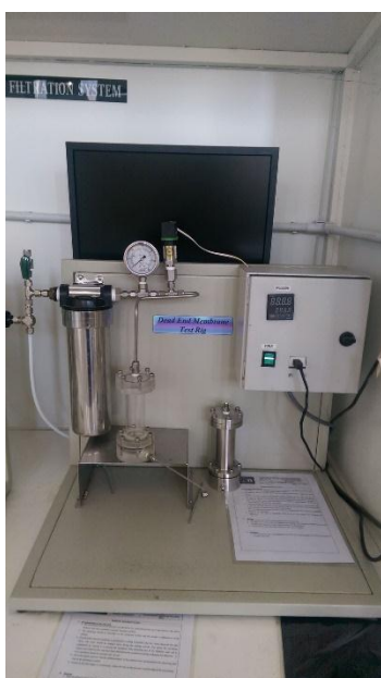
Dead End Filtration System
