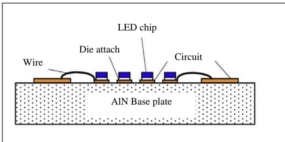
Figure 2.11: LED Module with AlN Base Substrate
