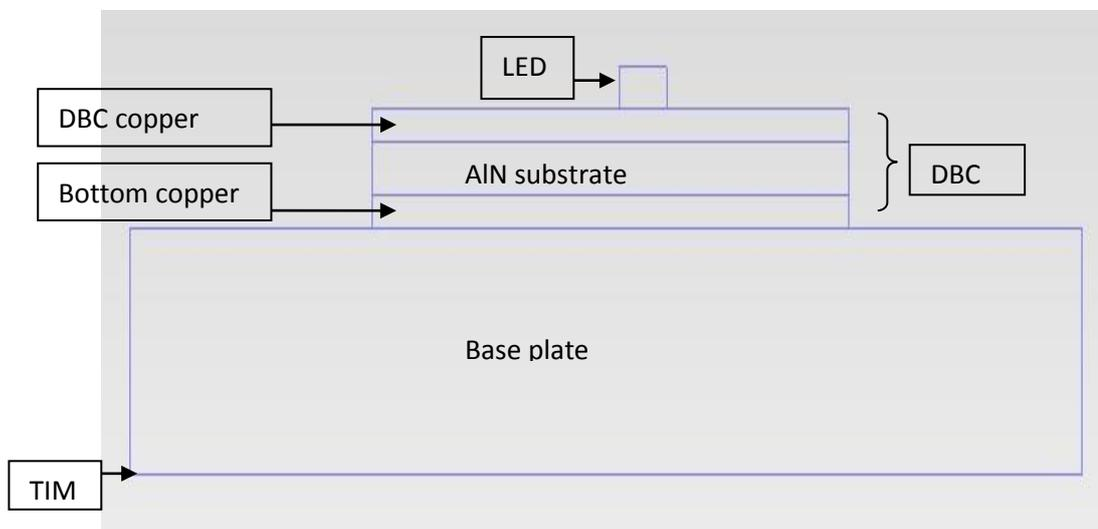
Figure 3.13: LED Module with DBC Substrate Design Layout
