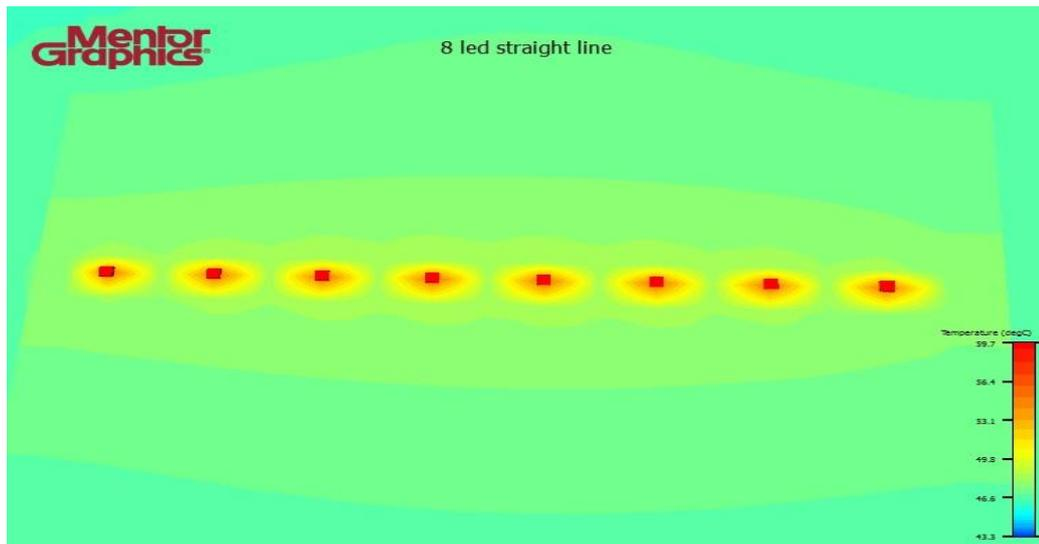
Figure 4.16: Simulation Result of Eight Multiple-Chips LED Module with Straight Line Orientation
