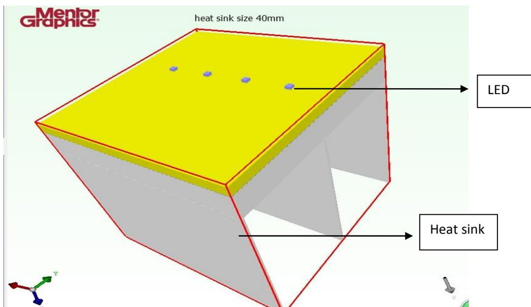
Figure 3.21: 3D view of the LED Module
