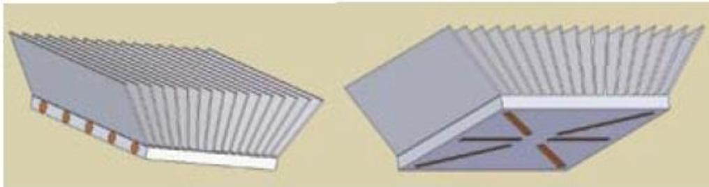
Figure 5.2: Embedded and Surface Embedded Heat Pipe Heat Sinks
