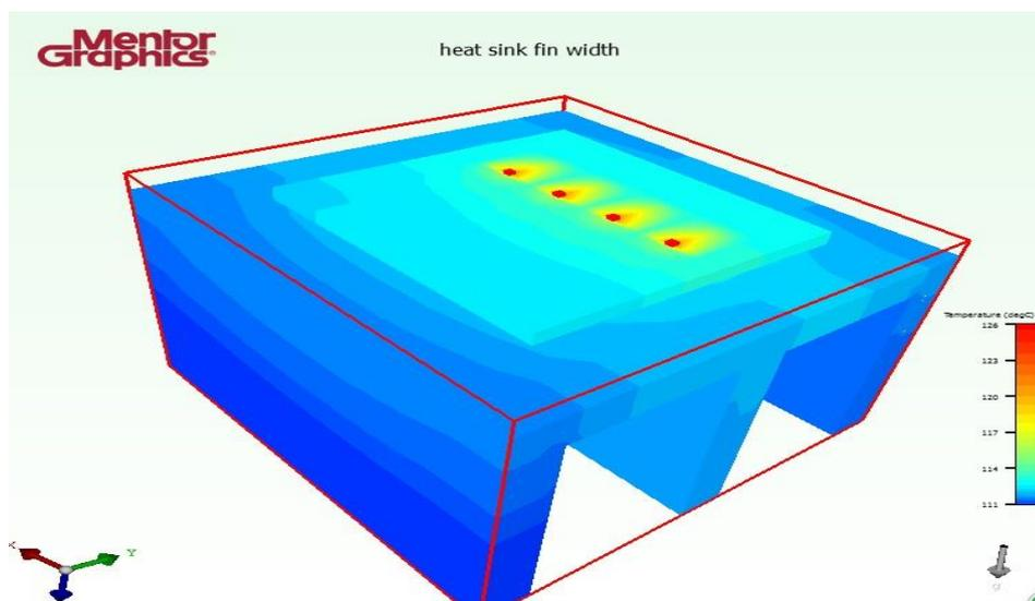
Figure 4.36: Result of LED Module with Fin Width of 6mm
