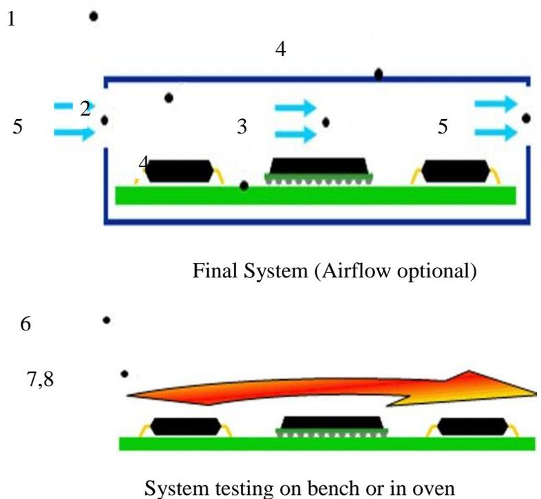
Figure 2.7: Eight Different Measuring Points for Ambient Temperature
