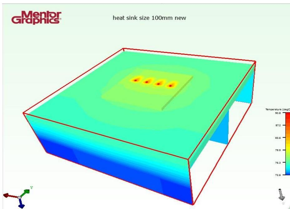
Figure 4.20: Result of LED Module with Area of 100 mm<sup>2</sup>
