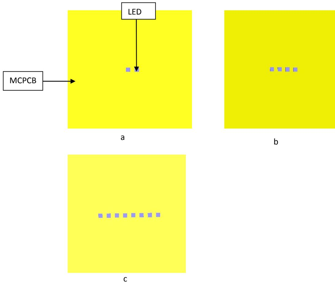
Figure 3.14: Z view of the LED module a) two LED chips module b) four LED chips module c) eight LED chips module
