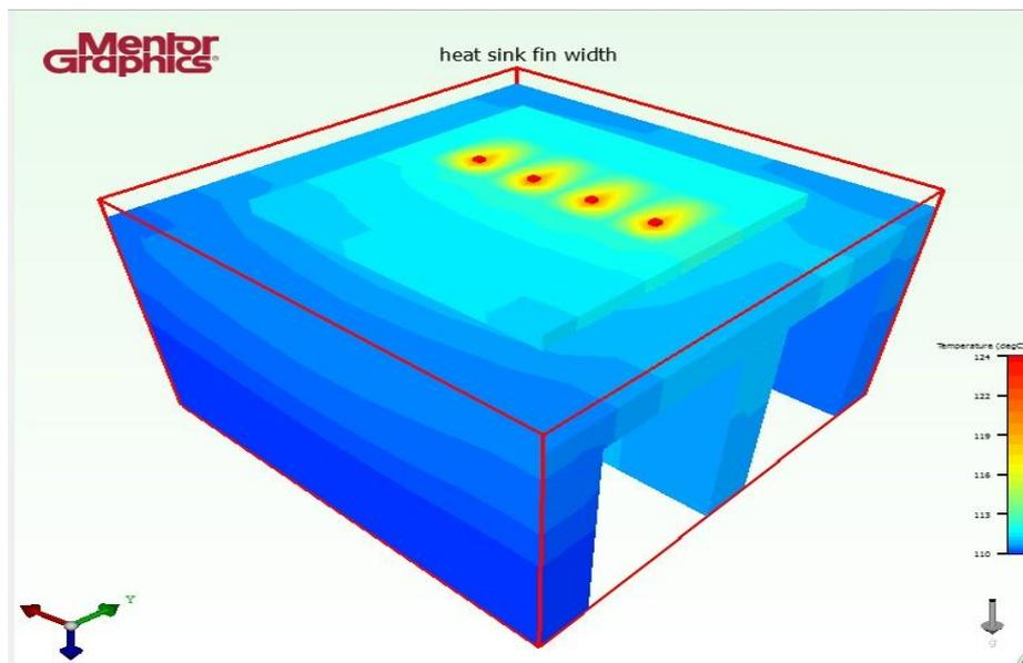
Figure 4.37: Result of LED Module with Fin Width of 7mm
