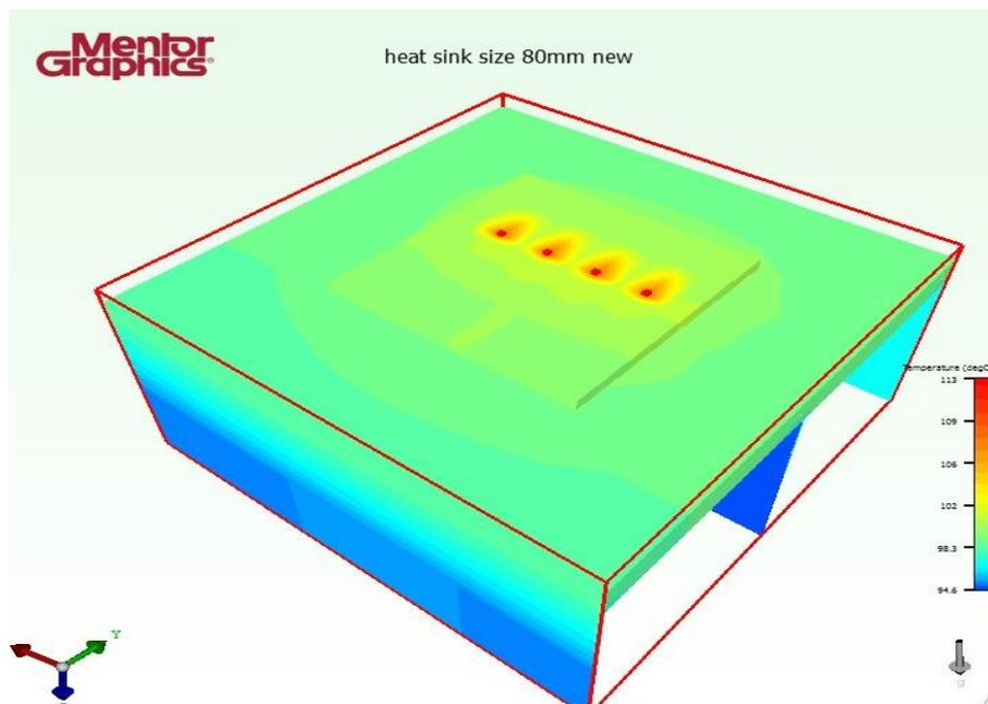
Figure 4.19: Result of LED Module with Area of 80 mm<sup>2</sup>
