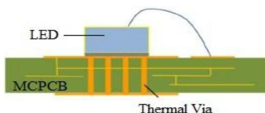
Figure 5.1: LED Module with Thermal Via
