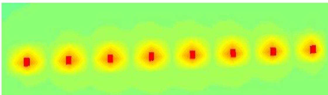
Figure 4.12: Simulation Result of Multiple-Chips LED Module with Distance between LED Chips of 8mm
