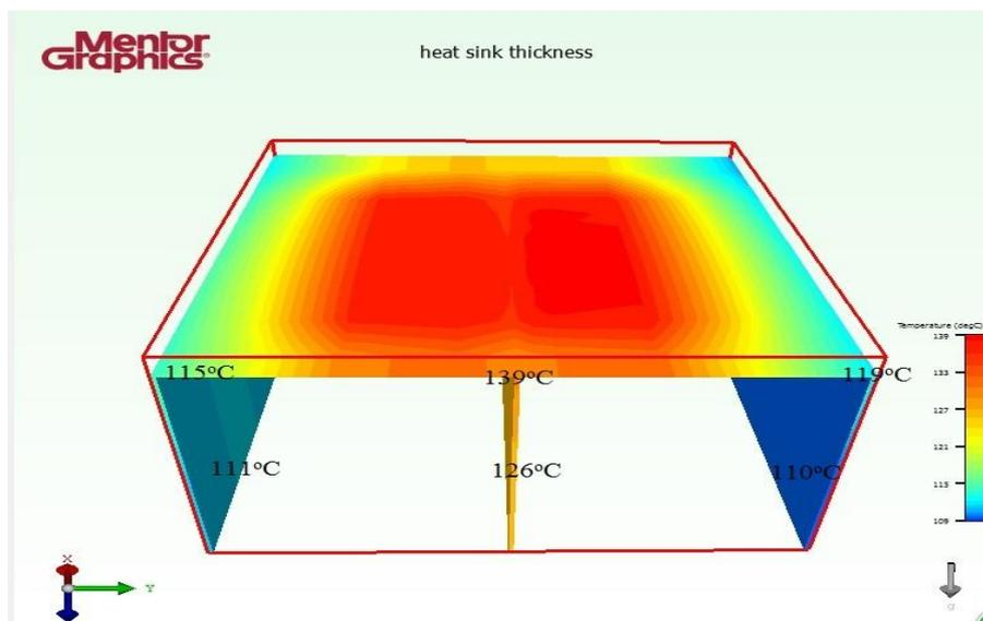
Figure 4.21: Result of LED Module with Thickness of 0.1mm
