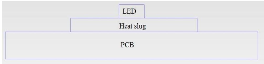
Figure 3.5 LED module design layout
