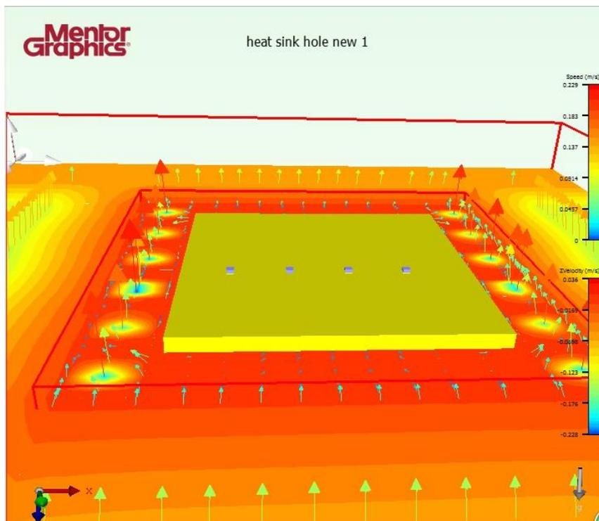
Figure 4.42: Velocity Map of the Heat Sink with Venting Holes
