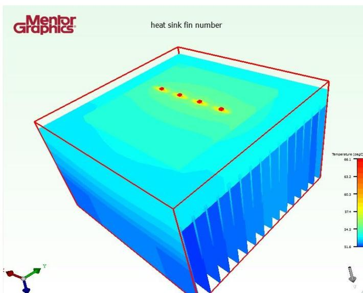
Figure 4.29: Result of LED Module with 16 Fins
