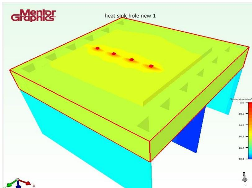
Figure 4.41: Result of LED Module with Venting Holes
