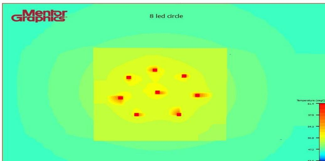
Figure 4.15: Simulation Result of Eight Multiple-Chips LED Module with Circle Orientation
