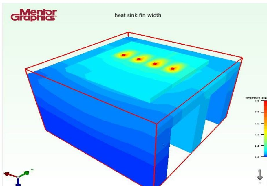
Figure 4.38: Result of LED Module with Fin Width of 8mm
