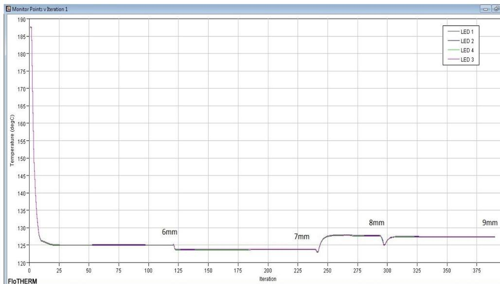
Figure 4.39: Graph of Temperature Versus Fin Width
