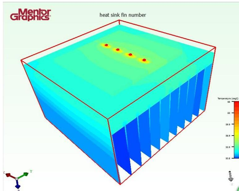
Figure 4.27: Result of LED Module with 11 Fins
