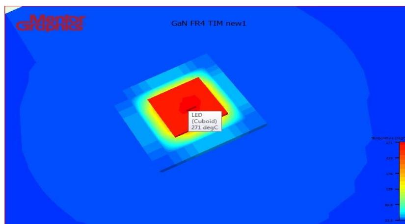
Figure 4.4: Result of GaN LED Chip Module with TIM Added
