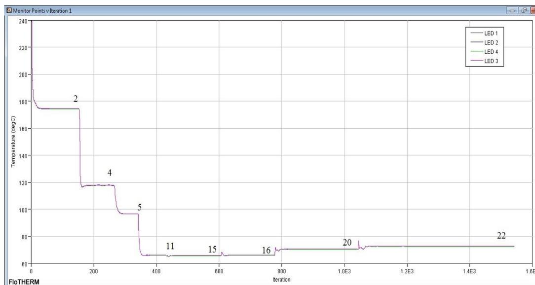
Figure 4.32: Graph Temperature Versus Fin Number
