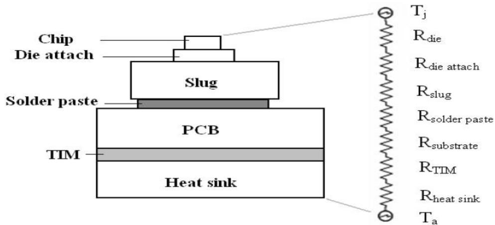
Figure 2.3: Thermal Resistance Found in a LED Module
