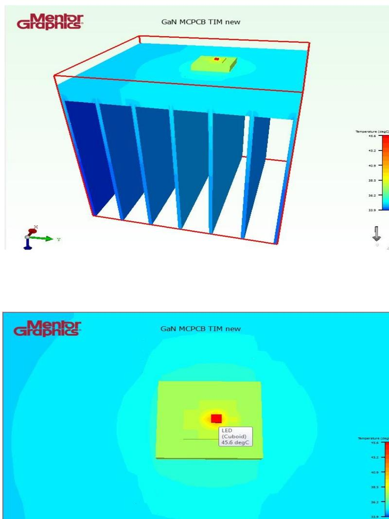
Figure 4.6: Result of GaN LED Module with MCPCB Substrate
