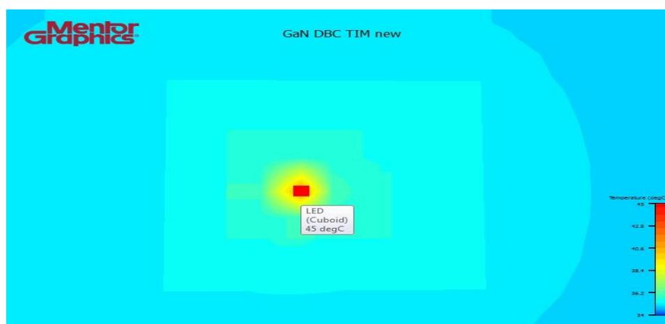
Figure 4.7: Result of GaN LED Module with DBC substrate
