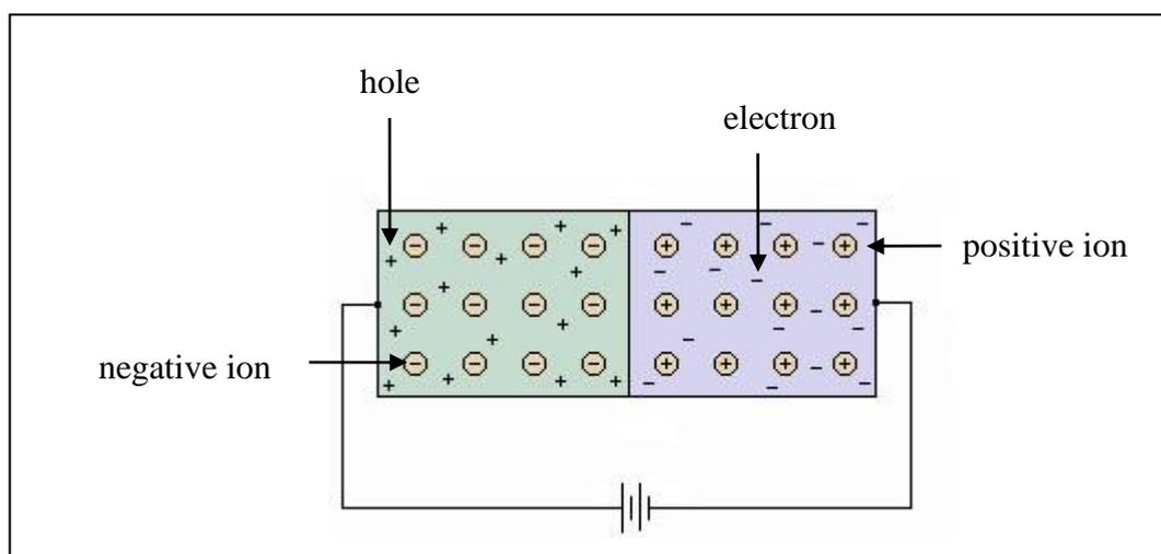
Figure 2.2: Forward Biased P-N Junction
