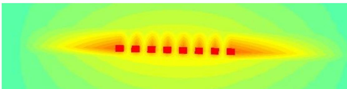
Figure 4.11: Simulation Result of Multiple-Chips LED Module with Distance between LED Chips of 2mm
