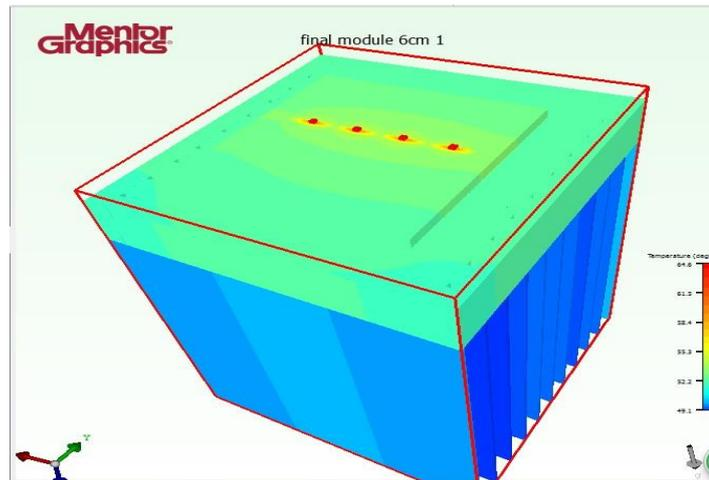
Figure 4.45: Thermal Distribution Map of the Optimized Multiple-Chips LED Module
