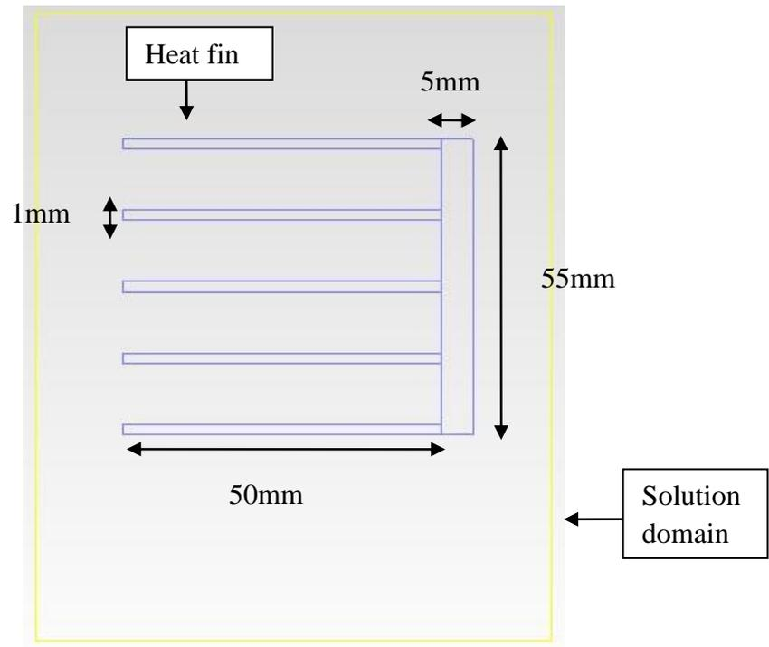
Figure 3.6: Heat Sink View on X Plane
