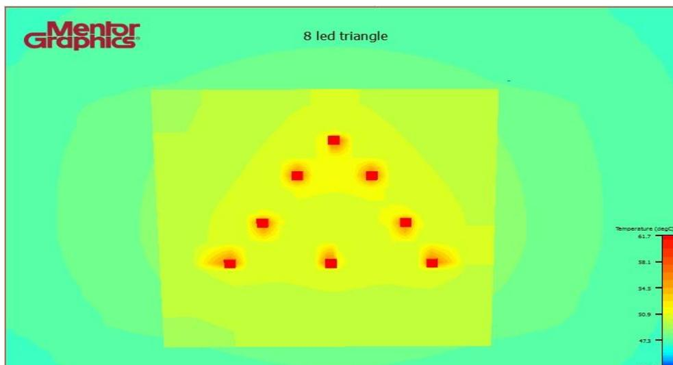
Figure 4.14: Simulation Result of Eight Multiple-Chips LED Module with Triangle Orientation
