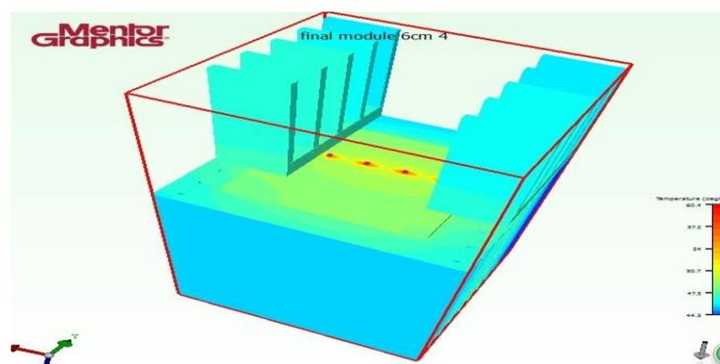
Figure 4.47: Thermal Distribution Map of Optimized Multiple-Chips LED Module with Additional Heat Sink
