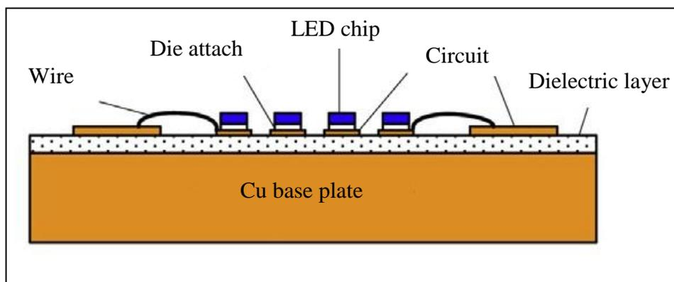
Figure 2.10: LED Module with Copper Base Substrate
