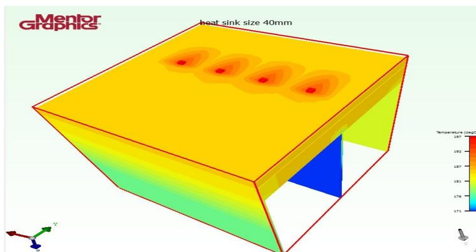
Figure 4.18: Result of LED Module with Area of 40 mm<sup>2</sup>
