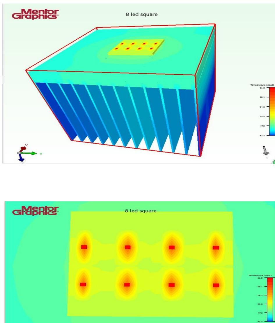
Figure 4.13: Simulation Result of Eight Multiple-Chips LED Module with Rectangle Orientation
