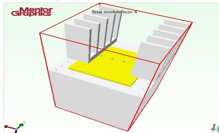
Figure 4.46: Optimized Multiple- Chips LED Module with Additional Heat Sink
