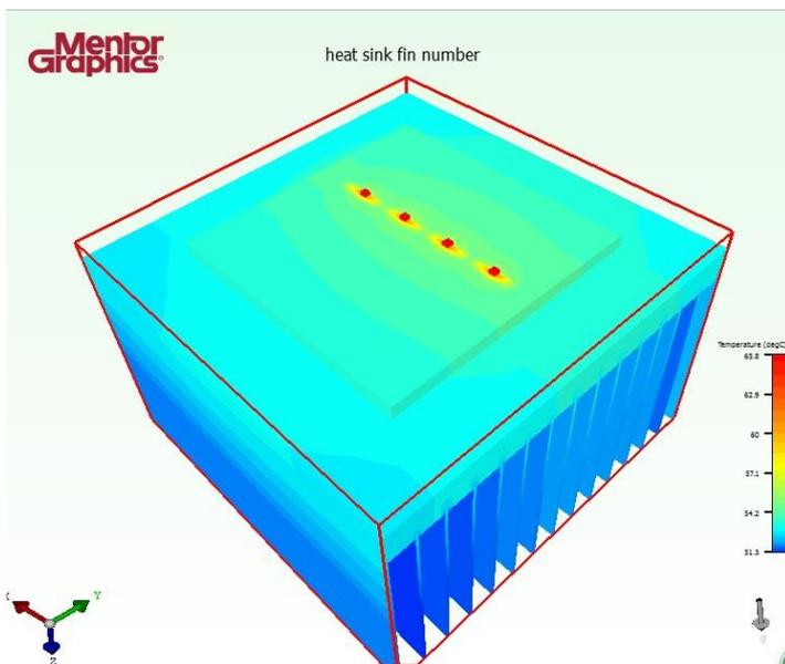
Figure 4.28: Result of LED Module with 15 Fins
