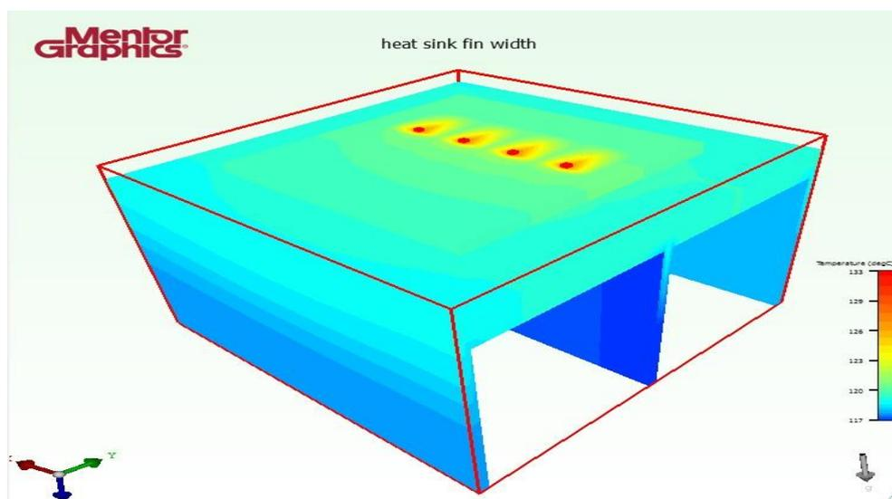
Figure 4.34: Result of LED Module with Fin Width of 1.5mm
