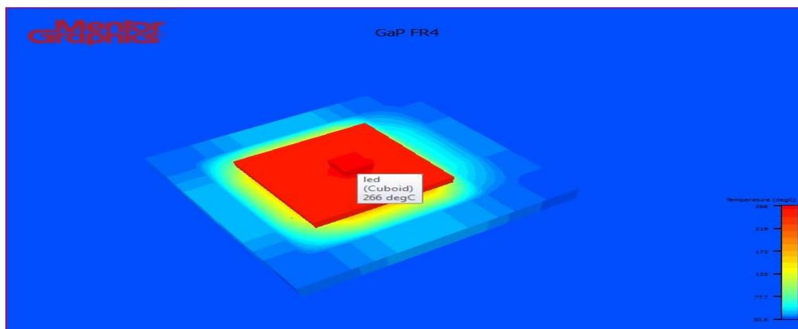
Figure 4.2: Result of GaP LED Chip
