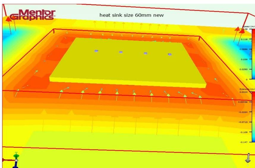
Figure 4.43: Velocity Map of the Original Heat Sink
