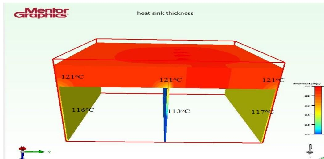
Figure 4.23: Result of LED Module with Thickness of 10mm
