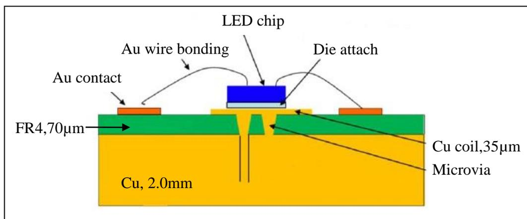
Figure 2.8: LED Module with Copper MCPCB with Vias
