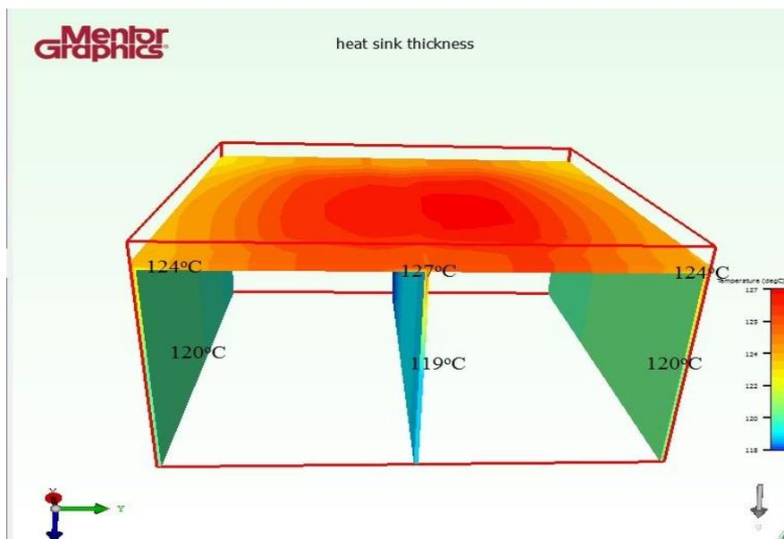
Figure 4.22: Result of LED Module with Thickness of 1mm
