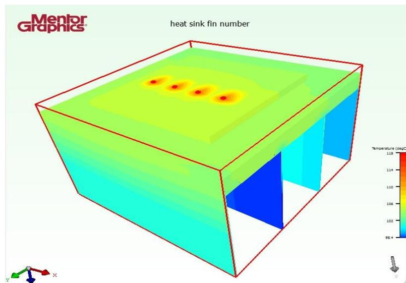
Figure 4.25: Result of LED Module with 4 Fins
