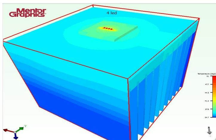
Figure 4.9: Multiple-Chips LED Module with four LED Chips
