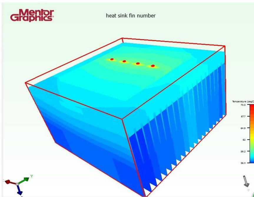
Figure 4.30: Result of LED Module with 20 Fins
