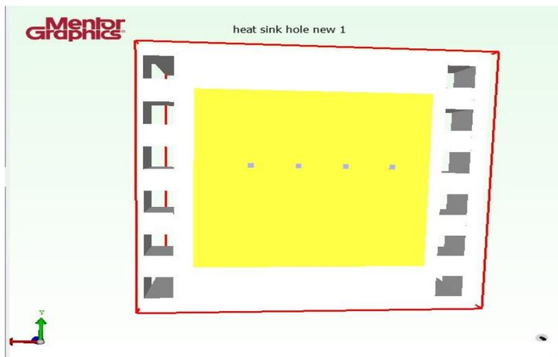
Figure 4.40: Heat Sink with Venting Holes
