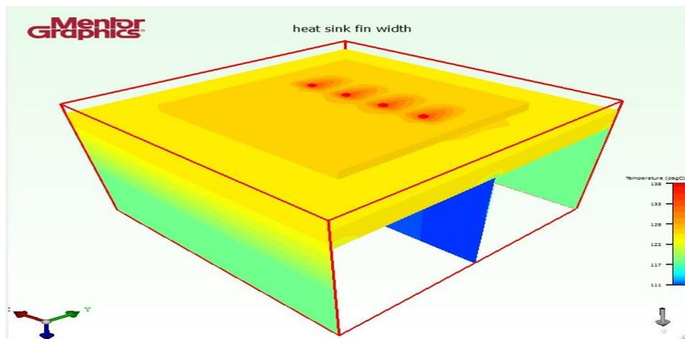
Figure 4.33: Result of LED Module with Fin Width of 0.25mm
