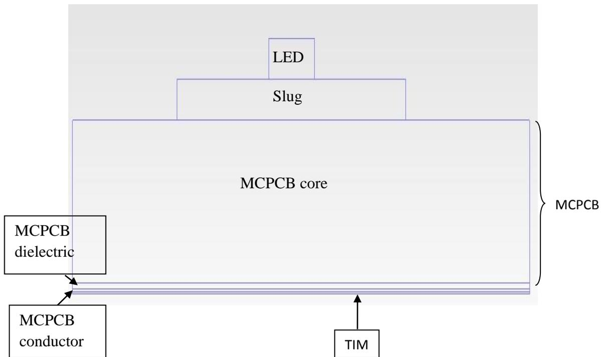
Figure 3.12: LED module with MCPCB Substrate Design Layout
