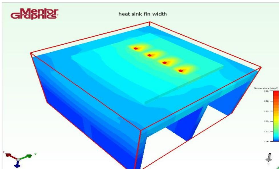
Figure 4.35: Result of LED Module with Fin Width of 3mm
