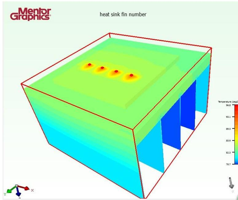
Figure 4.26: Result of LED Module with 5 Fins
