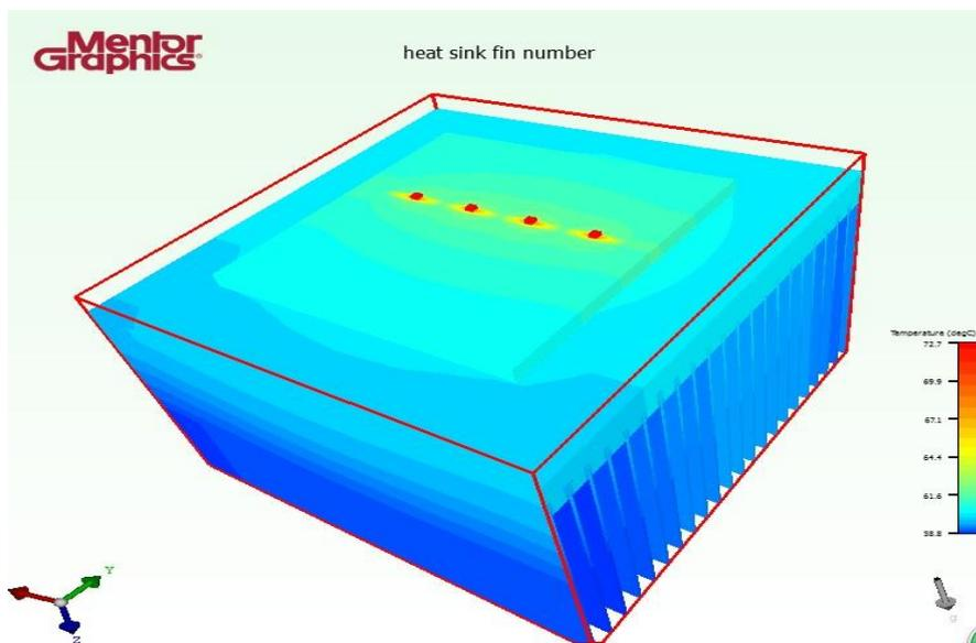
Figure 4.31: Result of LED Module with 22 Fins
