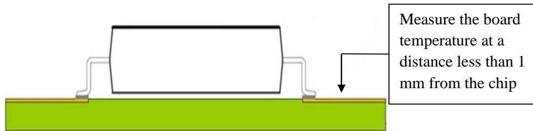
Figure 2.4: Ideal Measuring Point for Board Temperature
