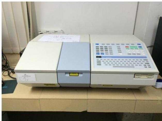
Figure 3.3: A Perkin Elmer RXI-IR spectrophotometer
