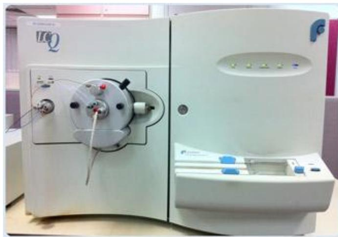
Figure 3.6: A Thermo Finnigan LCQ benchtop quadrupole ion trap mass spectrometer (This figure was taken from NUS, 2015)
