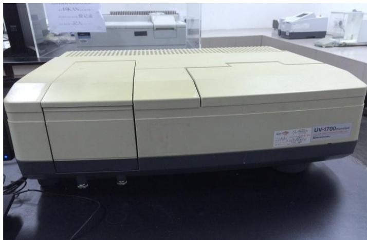
Figure 3.4: A Shimadzu UV-1700 UV-Visible spectrophotometer
