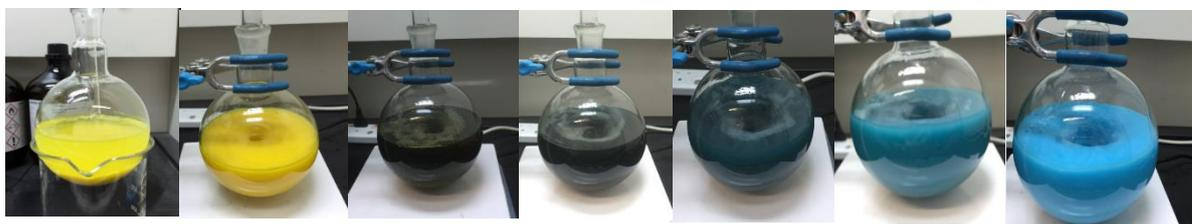
**Figure 3.2: Transition of Color during Reflux for Co-doped VPO**
