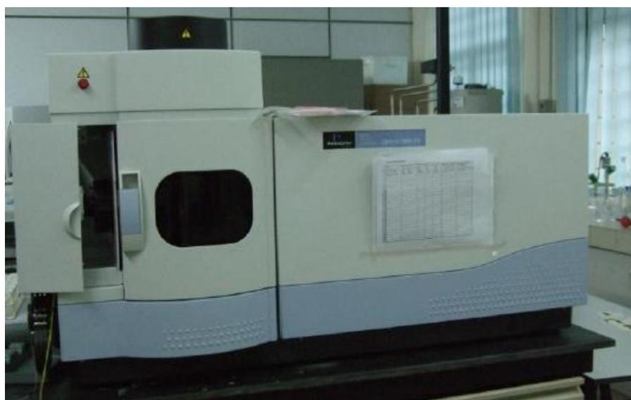
**Figure 3.11: Perkin Elmer Optical Emission Spectrometer Optima 7000 DV**
