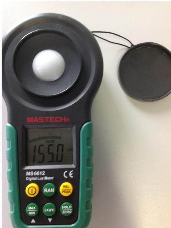
**Figure 4.25: Lux meter for measuring light intensity**
