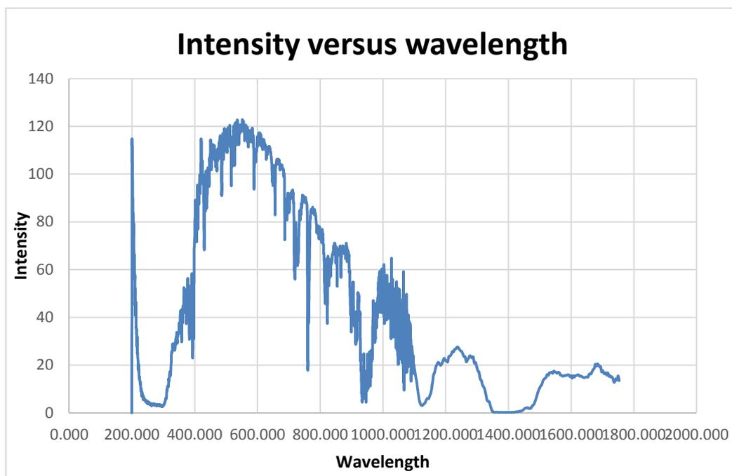
**Figure 4.1: Intensity of sunlight before hot mirror.**
