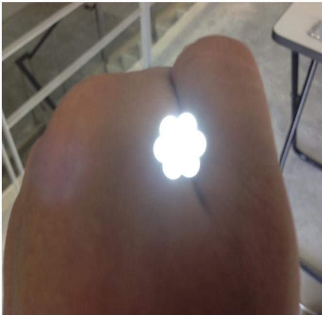
**Figure 4.19: one bundle of arranged in a hexagon like shaped.**
