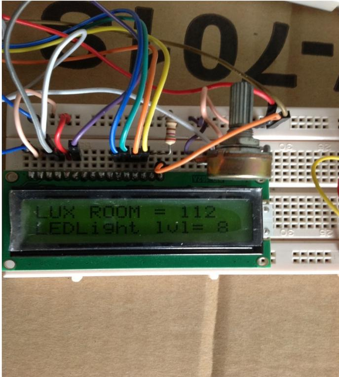
**Figure 4.17: LCD showing the lux of a room and led bright level**
