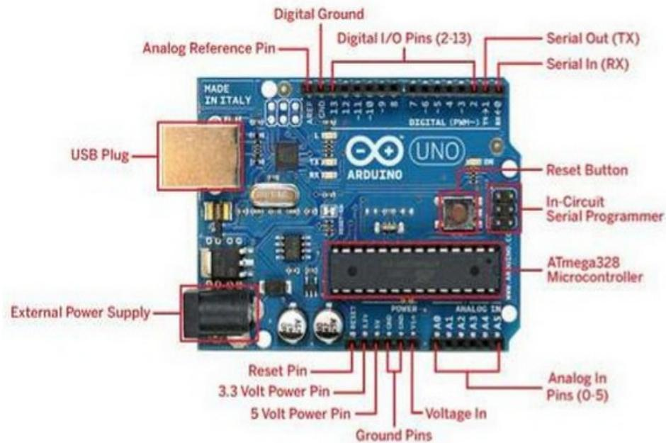
**Figure 3.23: Arduino Uno R3 and the pin mapping**
