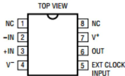
**Figure 3.30: LTC1050 operational amplifier and its pinout**
