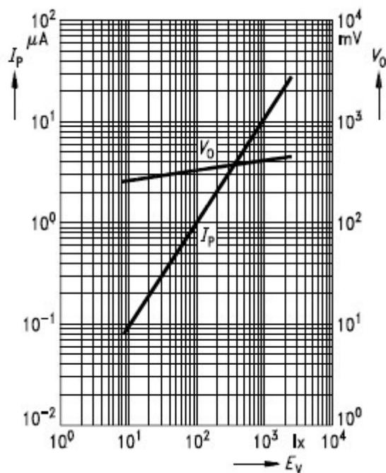
**Figure 3.29: Transfer Characteristic of BPW21**
