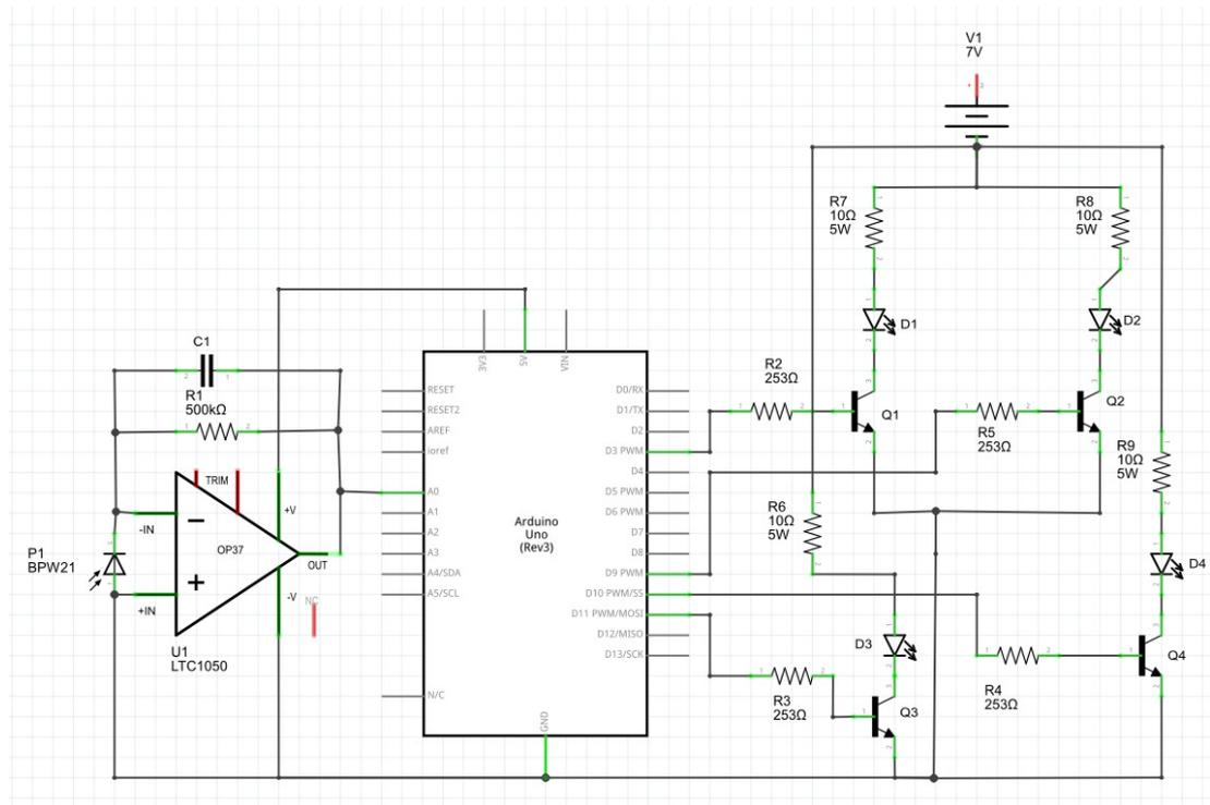
**Figure 3.34: Schematic drawing for the transistor amplifier circuit and photodiode sensor.**
