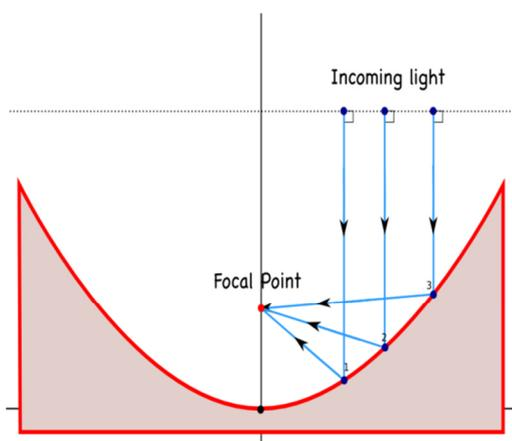
**Figure 2.4: Idea of Parabolic Reflector**
