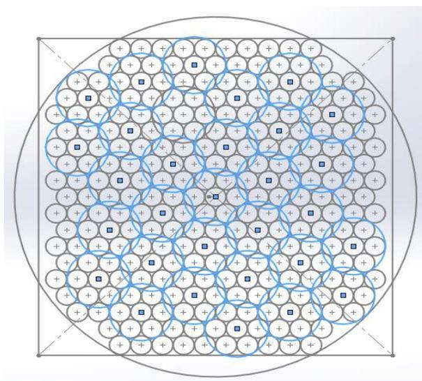
**Figure 3.18: Bundles of optical fiber for 5x5cm target**
