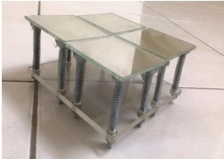
**Figure 3.2: Single assembly set of flat mirror as first stage of reflector**
