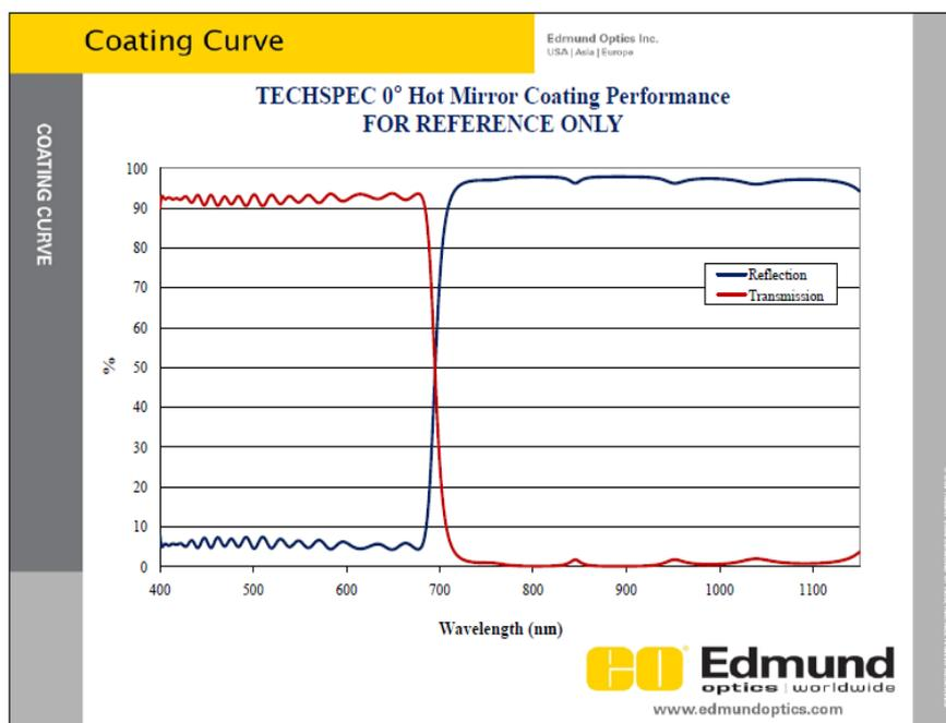
**Figure 3.11: Coating specification of the hot mirror**
