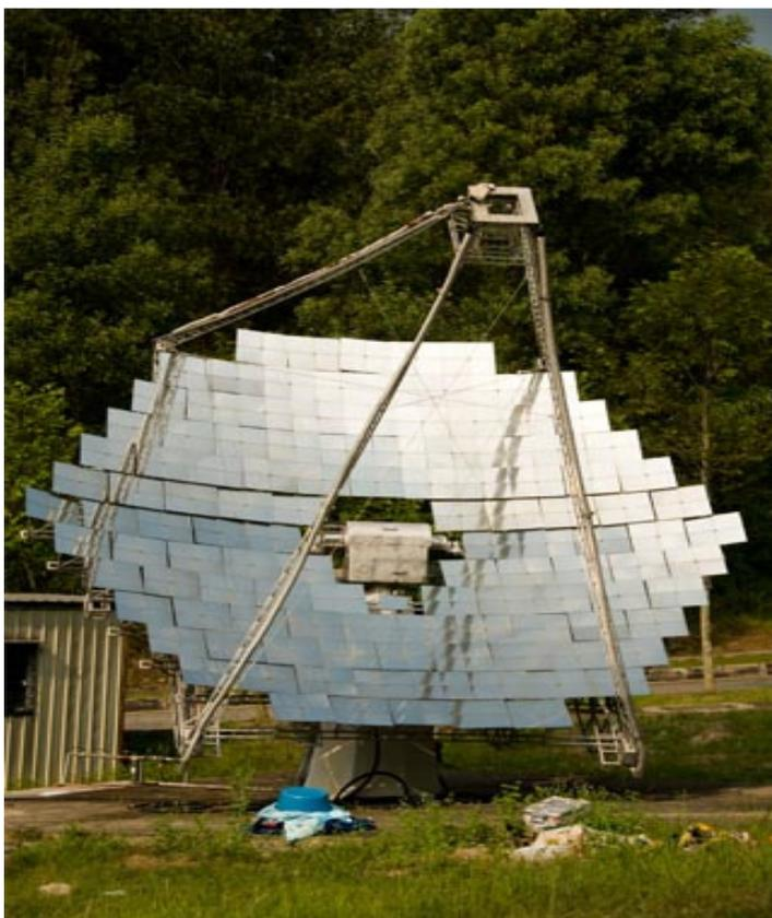
**Figure 2.6: Non-Imaging Dish Concentrator**
