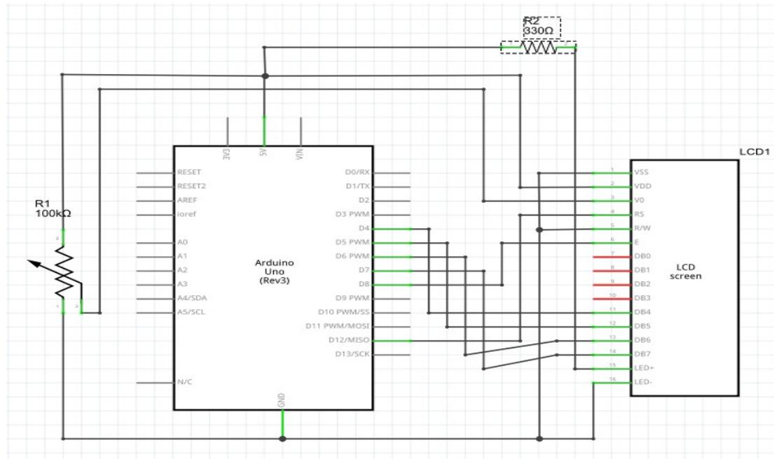
**Figure 3.26: Schematic circuit for LCD with Arduino Uno.**
