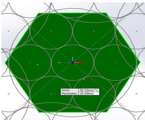
**Figure 3.36: Area of a bundle of optical fiber.**
