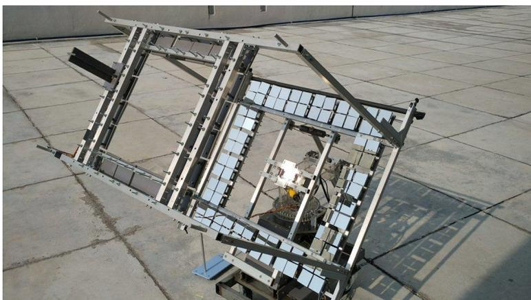
**Figure 4.22: working prototype of two-stage dish concentrator**
