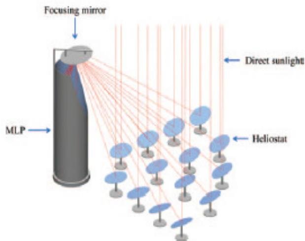
**Figure 2.1: Reflection of sunlight using heliostat**
