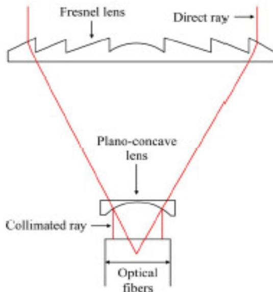
**Figure 2.5: Concept of Fresnel Lens**
