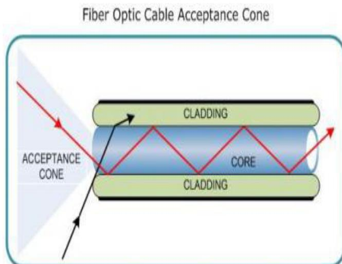
**Figure 3.7: Description of the acceptance cone on the light rays**
