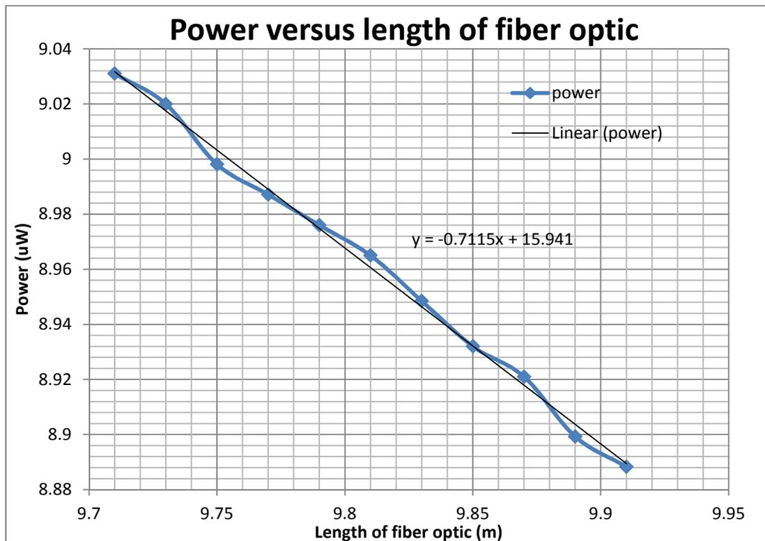
**Figure 4.5: Power versus length of fiber optic**
