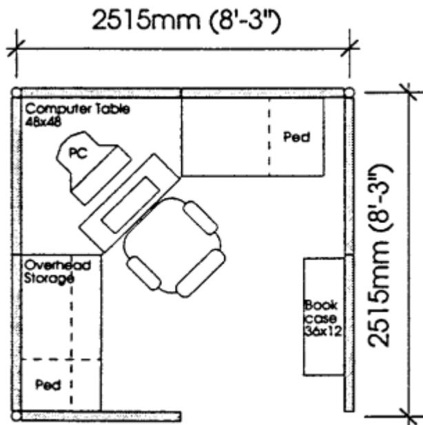
**Figure 3.40: Dimension and plan for standard office (6.5m<sup>2</sup>).**
