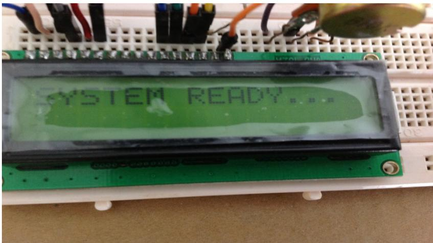
**Figure 4.15: Indication of system setting up**
