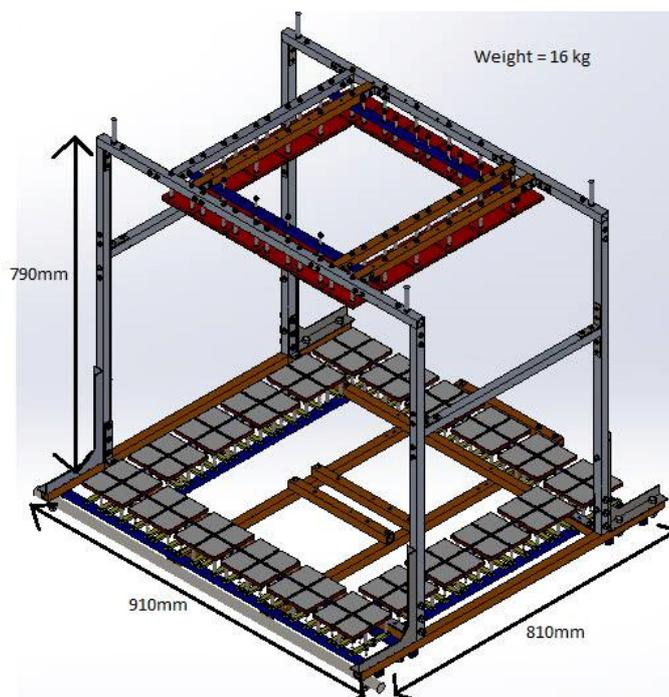
**Figure 3.3: Two-stage reflection using SOLIDWORKS**
