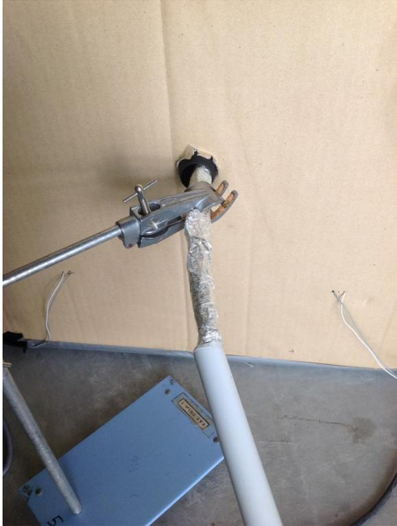
**Figure 4.23: The optical fiber was clamped with a retort stand to fix the position.**
