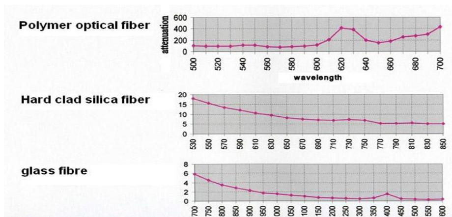
**Figure 2.7: Attenuation vs Wavelength of fiber optic**
