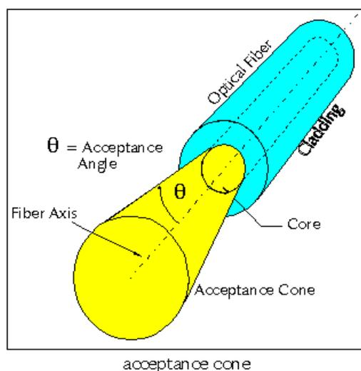
**Figure 3.6: Acceptance angle for the optical fiber**
