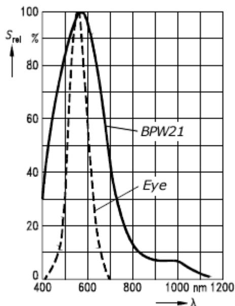
**Figure 3.28: Relative Spectral Sensitivity of bpw21**
