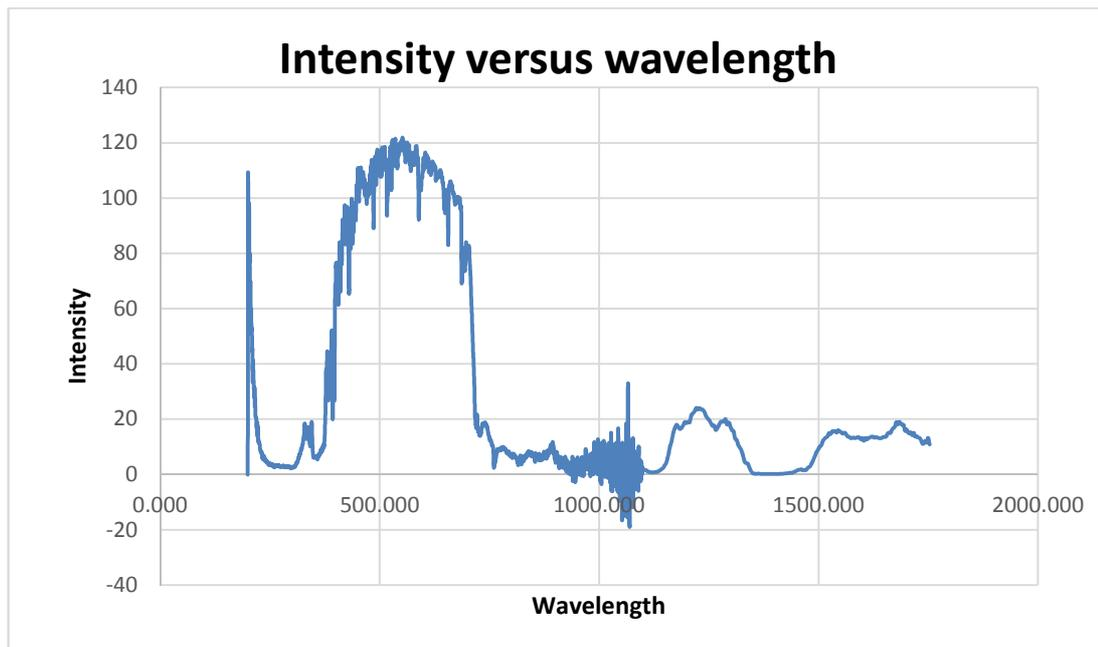
**Figure 4.2: Intensity of sunlight after the hot mirror**
