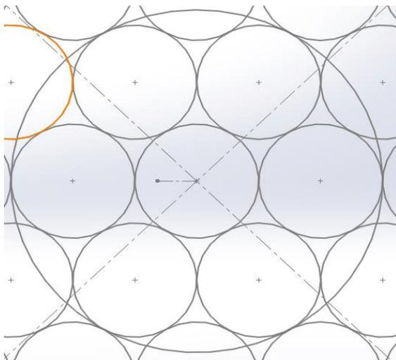
**Figure 3.17: A bundle consist of seven optical fiber**
