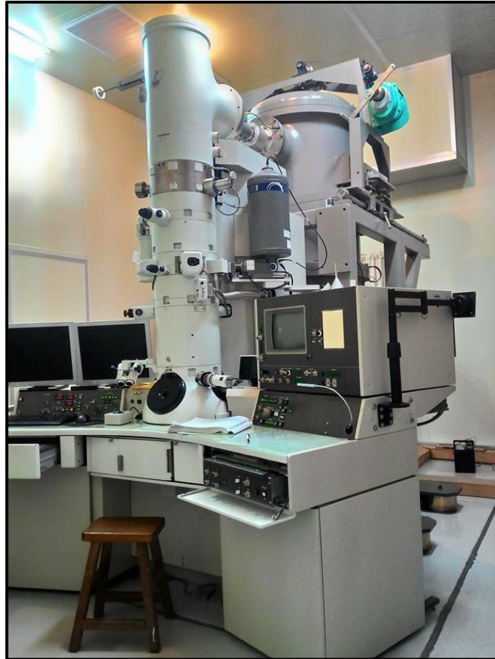
Figure 3.2: HRTEM (JEOL, JEM-3000F, 300 kV).
