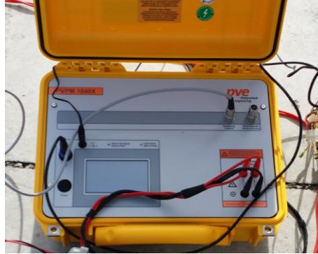
Figure 3.5: Solar analyser PVPM 1040X
