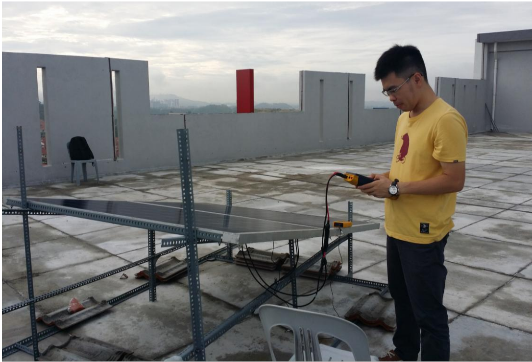
Figure 3.7 : Power and irradiance measurement taken by Seaward meter
