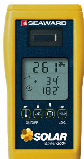
Figure 3.5 : Seaward S200R Solarimeter
