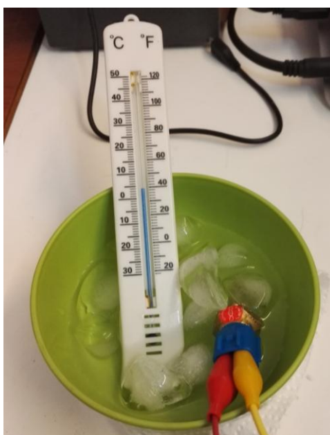
Figure 4.12: Measurement method of CTS
