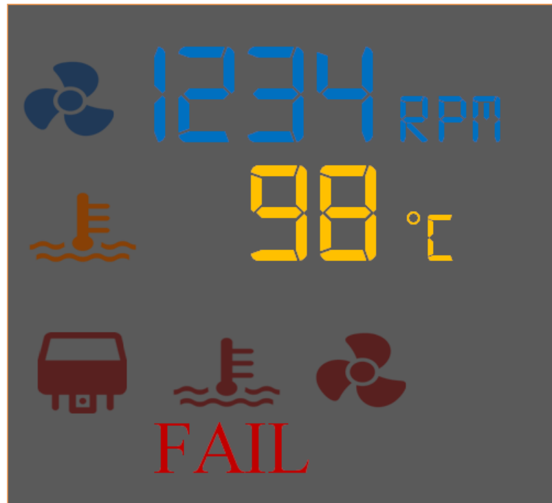
Figure 3.13: Cooling fan failure alert system display
