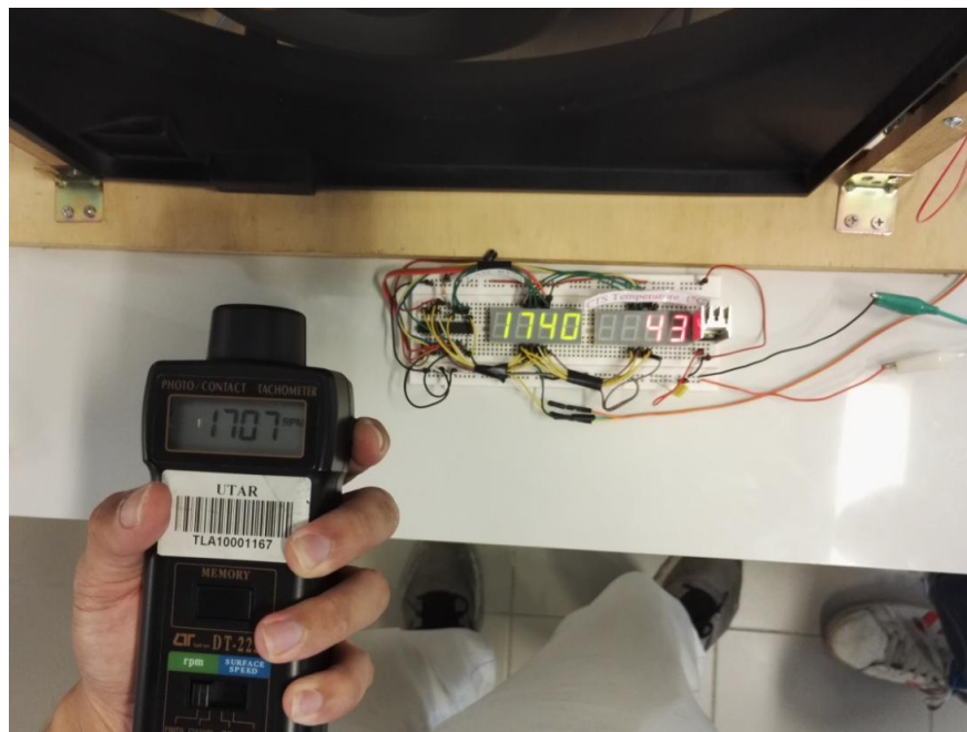
Figure 4.11: Measurement of Tachometer and Hall Effect sensor (Green LED)
