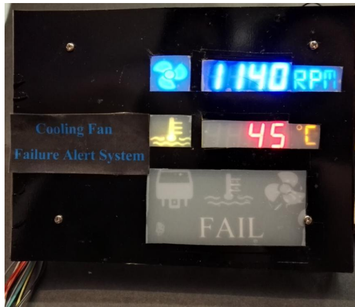
Figure 4.14: Cooling fan failure alert system display
