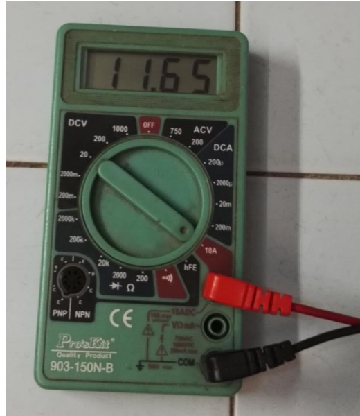
Figure 4.8: Multimeter measured starting current
