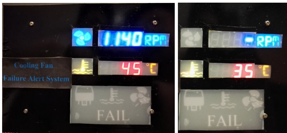
Figure 4.15: Cooling fan ON (Left) and OFF (Right)
