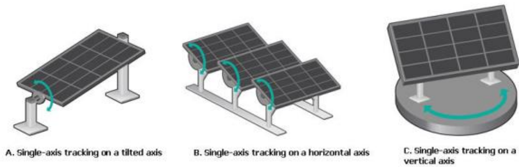
Figure 2.4: Types of One-Axis Tracker (Chuck Juda, 2013)
