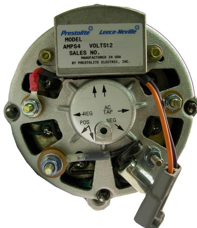
Figure 2.2: Alternator with AC tap output as indicated by the sticker label (Prestolite, n.d)
