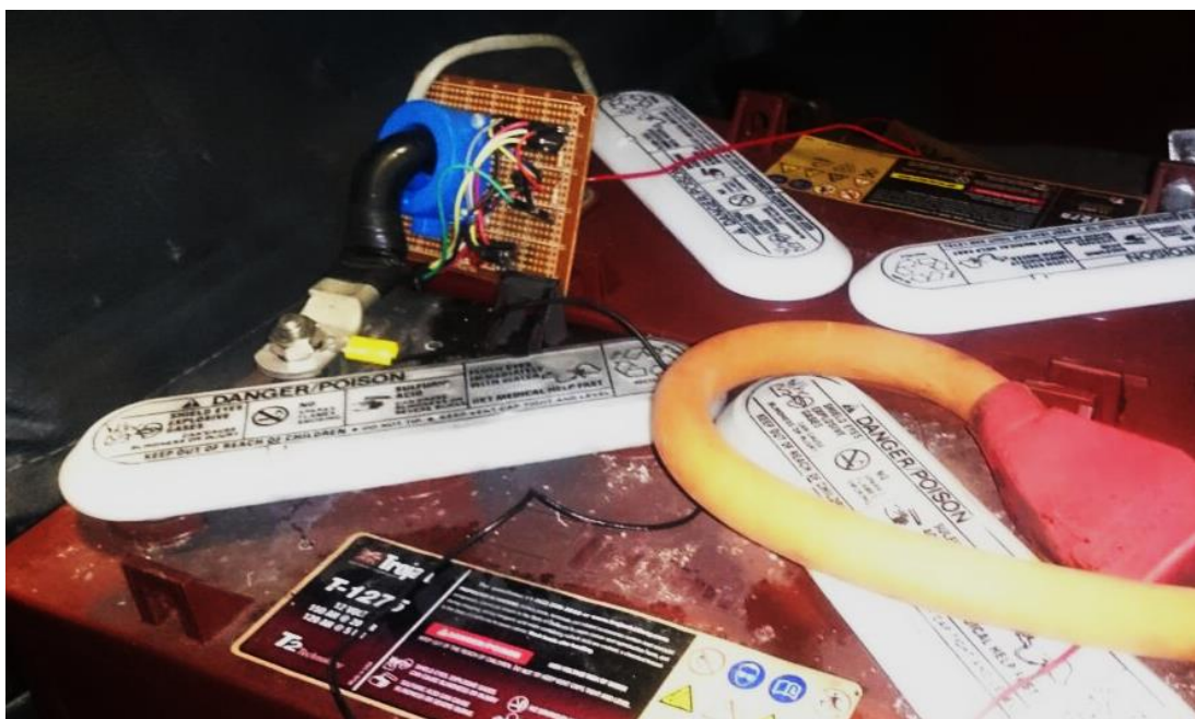
Figure 3.2: The existing LEM current sensor installed in the UTAR electric vehicle
