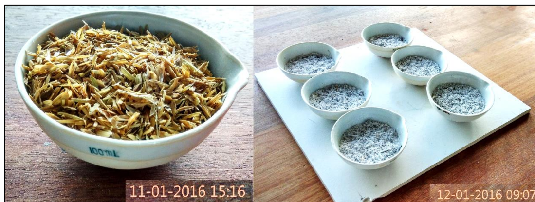
Figure 3.3: Transformation of Rice Husk into Ash
