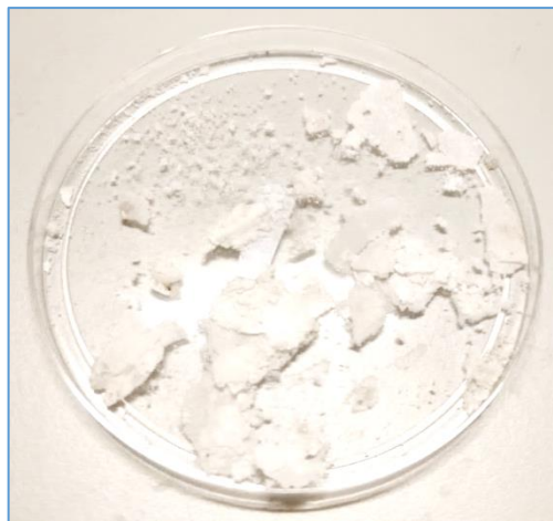
Figure 4.23: Calcium Carbonate Precipitate on Cement Cubes
