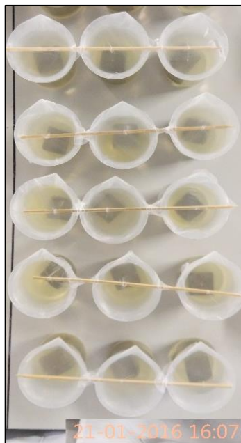
Figure 3.1: Cement Cube Samples in Contact with Acetic Acid
