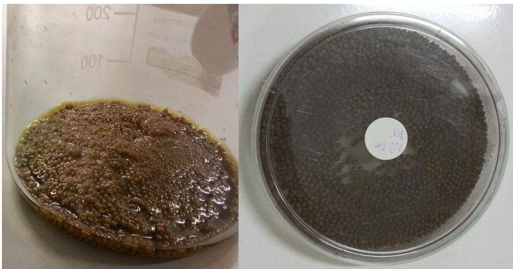
Figure 4.3: Catalyst synthesised by dry impregnation method before drying (left) and after calcination (right).
