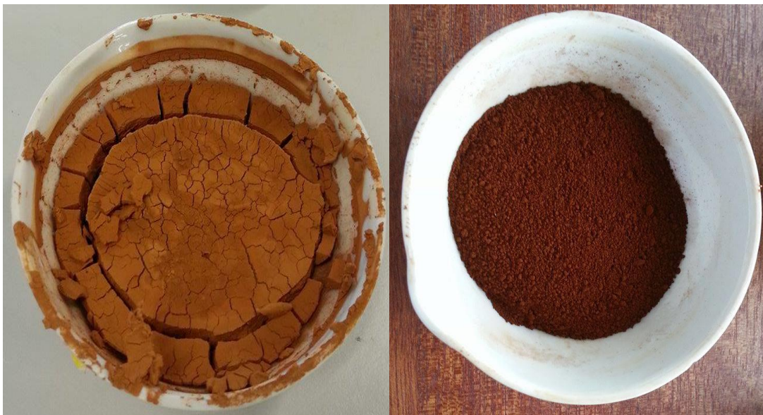
Figure 4.4: Catalyst synthesised by co-precipitation method after drying (left) and after calcination (right).
